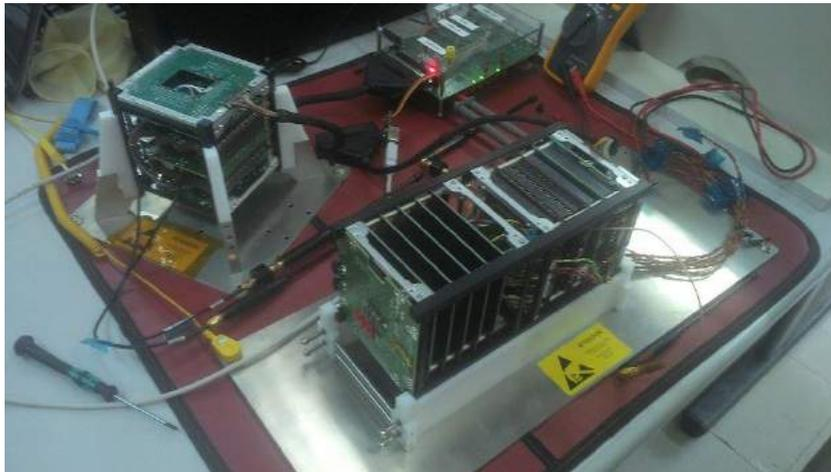
**Figure 4** – The NANOSATC-BR1 and NANOSATC-BR2 Engineering Model Platforms.
