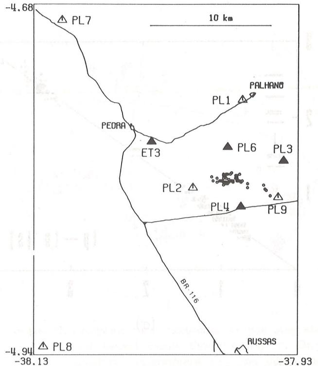
**Figure 3.** Distribution of fixed stations (solid triangles), moving stations (open triangles) and epicenters (dots). A maximum of five stations were operating at any time.
