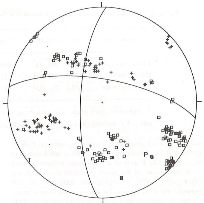
**Figure 7.** Composite focal mechanism solution using the best located events shown in Fig. 5. Only impulsive compressional (+) and dilatational (square) P-wave first motions were used. 'P' and 'T' are the pressure and tension axes respectively. Lower hemisphere equal-area projection.
