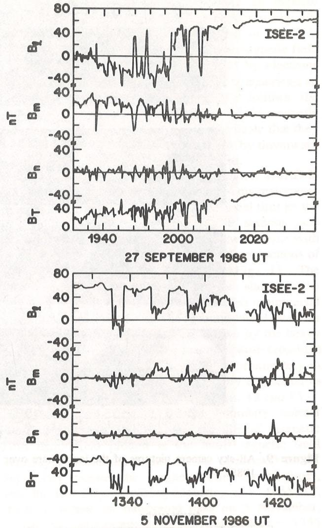
Figure 12. Magnetic field vectors as measured on ISEE-2 and expressed in boundary normal coordinates during the crossing of the magnetopause along the trajectories illustrated in Fig. 11.
