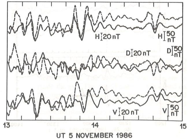
Figure 13. Time-intensity magnetic field data measured at IQ and SP during the ISEE-2 boundary crossing events of Fig. 12.
