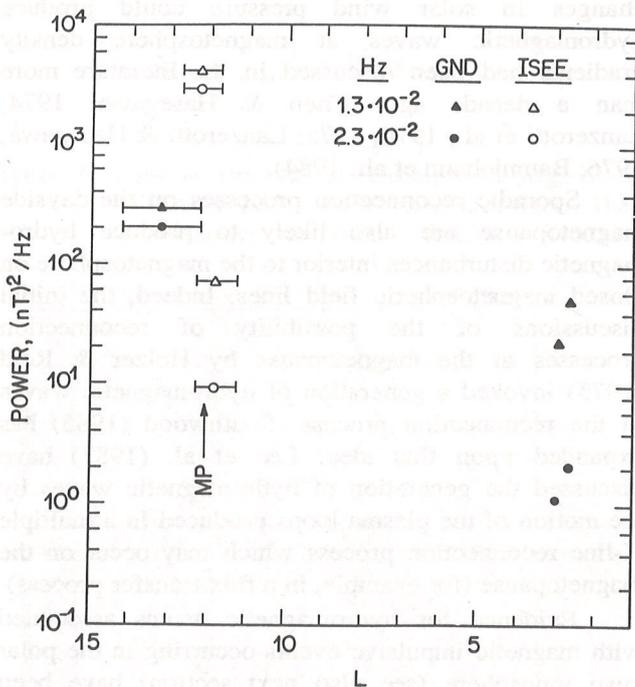
**Figure 2.** Power spectral levels of magnetic field fluctuations at two frequencies as measured on the ground and on the ISEE-2 spacecraft. Data are plotted as a function of L-value, although precise values near the magnetopause are uncertain and depend upon magnetosphere model used (Lanzerotti et al., 1989).
