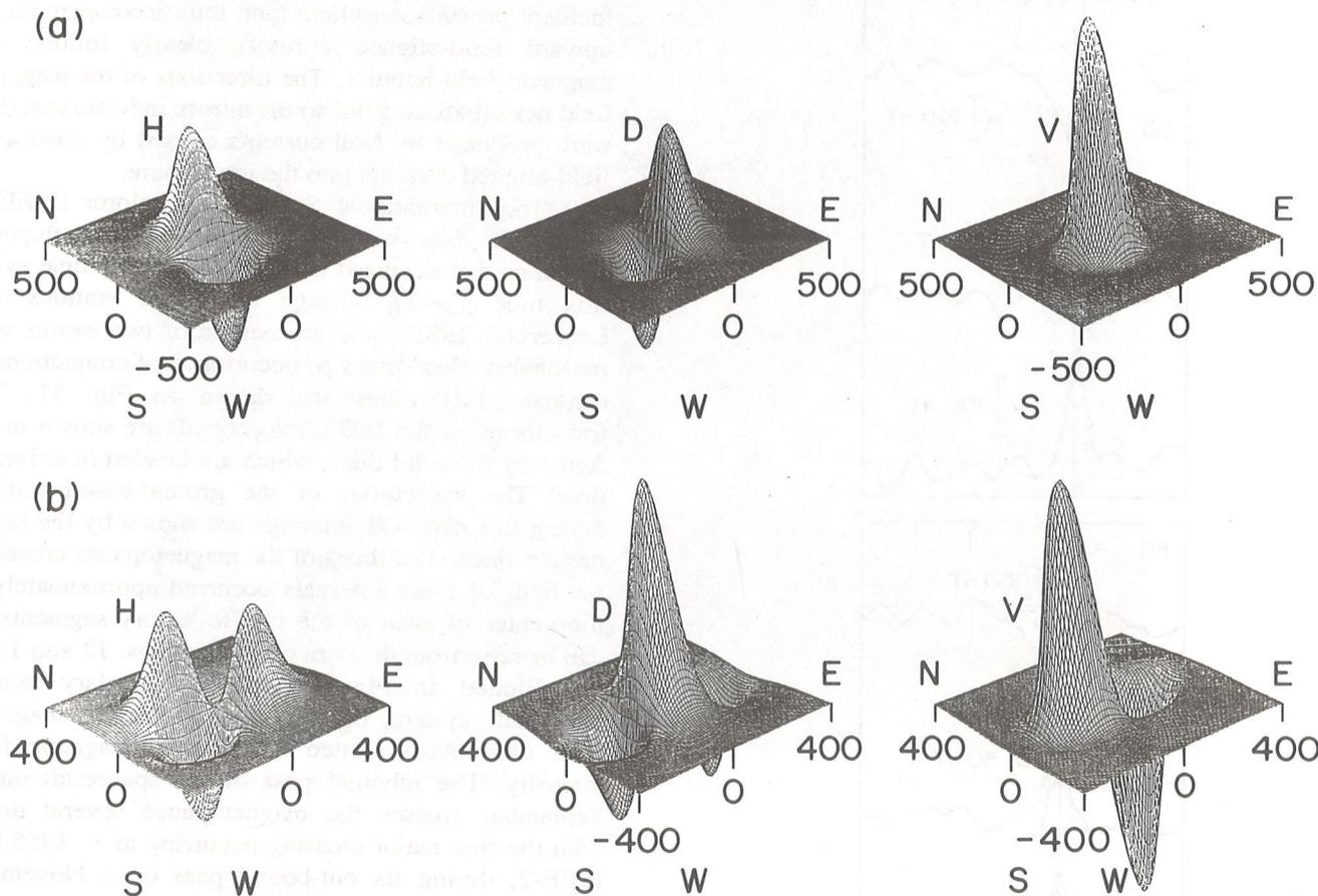
**Figure 7.** Spatial distribution of magnetic variations expected at the Earth's surface in three orthogonal directions (H: geomagnetic south-north; D: geomagnetic west-east; V: vertical, with positive vertical variation corresponding to a magnetic field increase in the direction of the main field) from the two Hall current patterns shown in Fig. 6.
