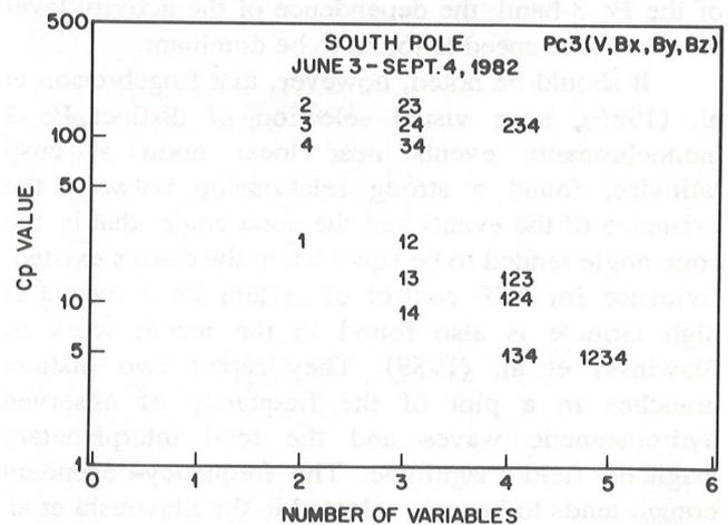
**Figure 3.** The value of the  $C_p$  statistic for a given number of variables ( $p$ ). The power in the Pc 3 frequency band is found to be most highly associated with solar wind speed  $V$  (variable number 1) and then with  $B_z$  (variable number 4). The  $B_x$  component (variable number 2) is found to be not significantly associated with the Pc 3 power.
