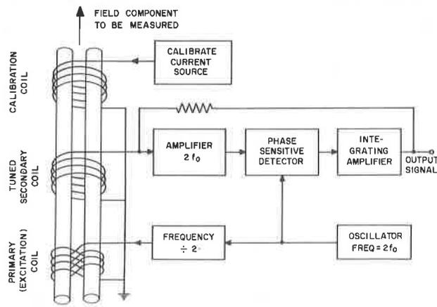
Figure 1 - Schematic block diagram of a fluxgate magnetometer.
