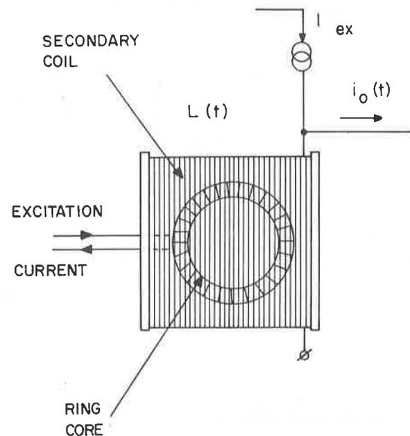
Figure 2 - Mechanical design of ring core sensor housing.
