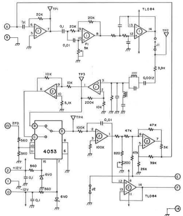
Figure 4 - Circuit diagram of amplifier and synchronous phase detection.
