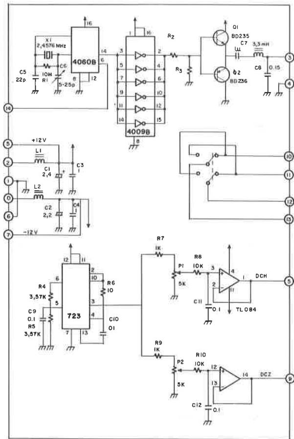
Figure 3 - Circuit diagram of oscillator and reference voltage
