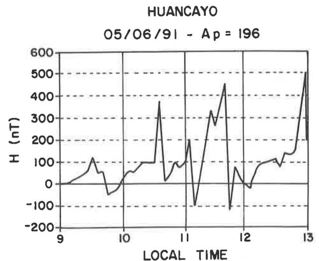
Figure 8 - Storm time variation in H during 09:00-13:00 hours L.T. on 5 June 1991 at Pimenta Bueno and Huancayo.
