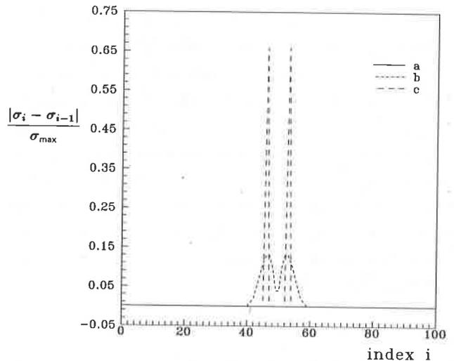
**Figure 3** - Normalized first-differences of models **a**, **b** and **c**, and respective first-order entropy values,  $\bar{S}_1^a = 1.000$ ,  $\bar{S}_1^b = 0.5958$  and  $\bar{S}_1^c = 0.1502$ .
