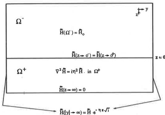
**Figure 1** - Geometry and boundary conditions of the forward problem.
