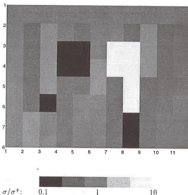
Figure 5 - Conductivity map in logarithmic scale;  $\gamma_0 = 0$  e  $\gamma_1 = 0.50$ , data with 8% gaussian noise (true model shown in Fig. 4a).
