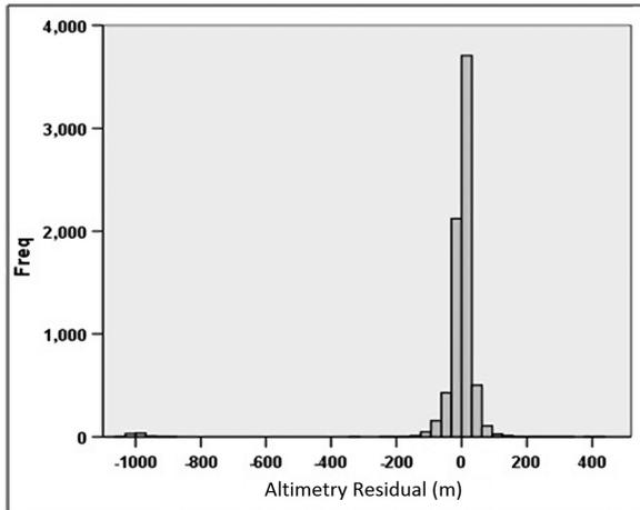
Figure 4 – Histogram of the differences between the elevation values of the 7.218 points and the respective SRTM points interpolated by the Krigagem method.
