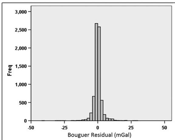
Figure 6 – Histogram of the differences between Bouguer anomaly values calculated from the 7.218 points and the respective Bouguer anomaly points interpolated by the Krigagem method.
