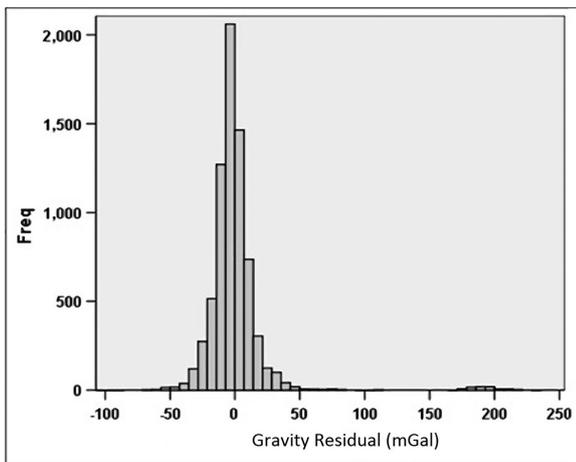
Figure 5 – Histogram of the differences between gravity values of the 7.218 points and the respective GRACE mission points interpolated by the Krigagem method.
