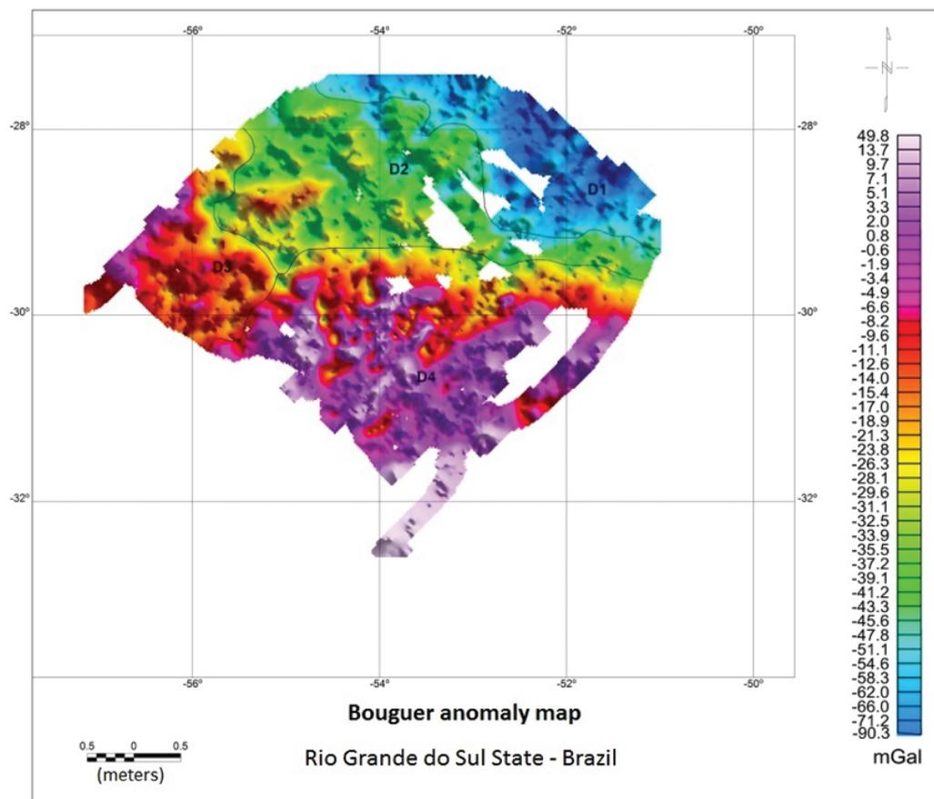
Figure 10 – Bouguer anomaly map of RS showing gravimetric domains, characterized from the corrected database.
