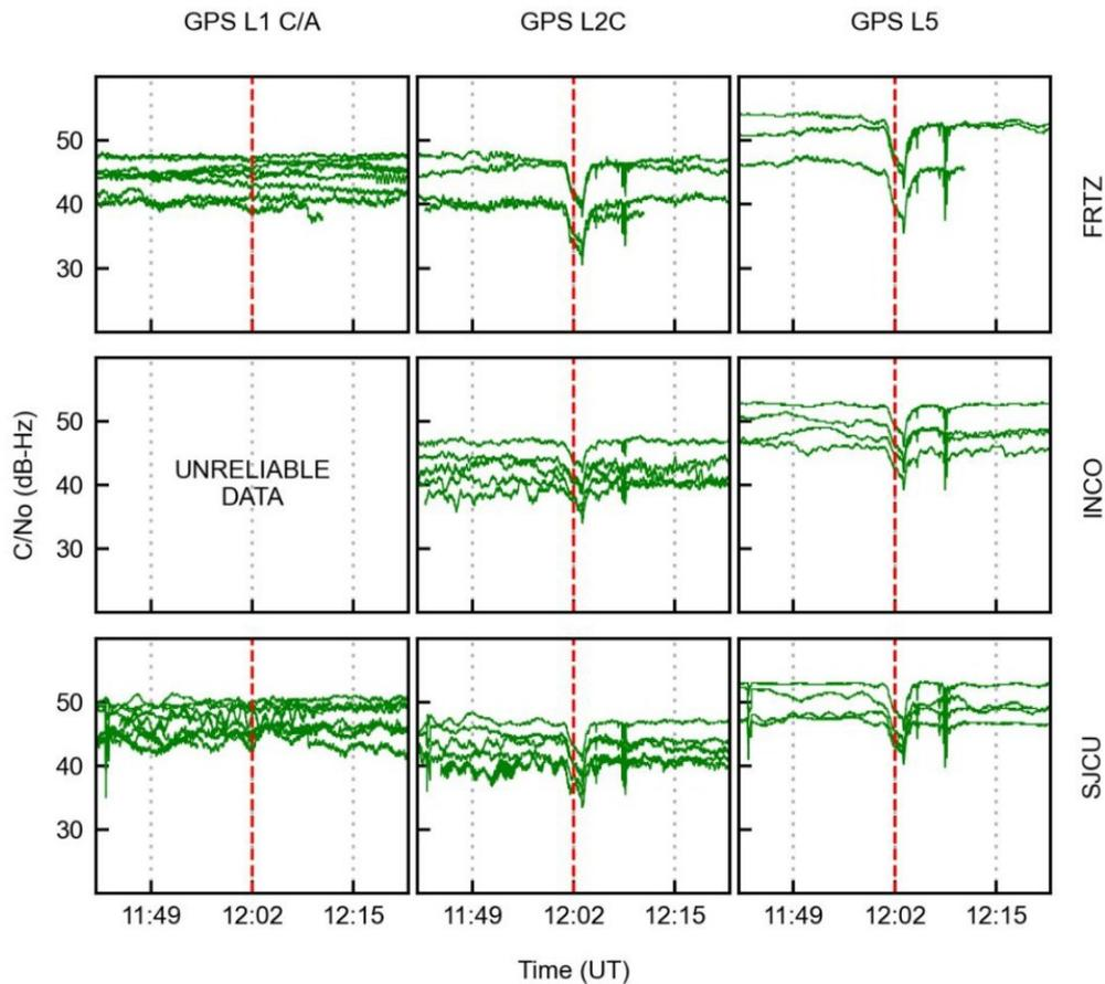
Figure 13: GPS C/No signal for L1, L2C and L5 GPS frequencies during 06 September 2017 for the sites FRTZ, INCO and SJCU. The vertical red line is the time of the solar flare maximum (source: [de Paula et al., 2022](#)).
