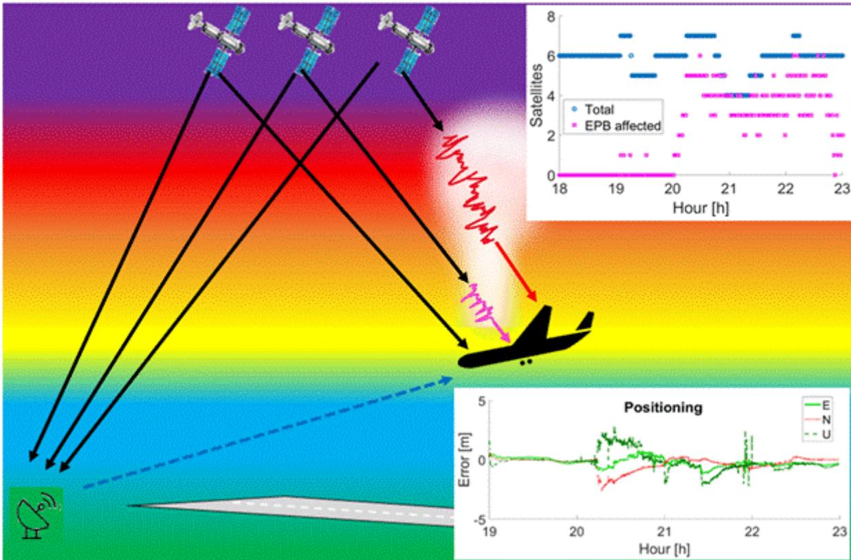
Figure 17: Pictorial example of an aircraft being affected by scintillation causing degradation in positioning accuracy (source: the authors).
