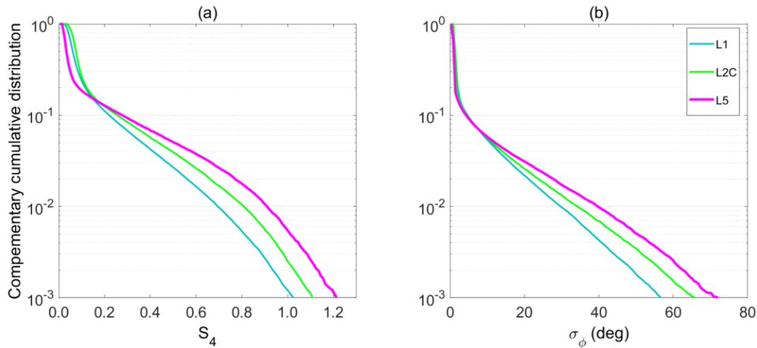
Figure 4: Complementary cumulative distributions of  $S_4$  and  $\sigma_\phi$  for the L1, L2C, and L5 signals (source: the authors).
