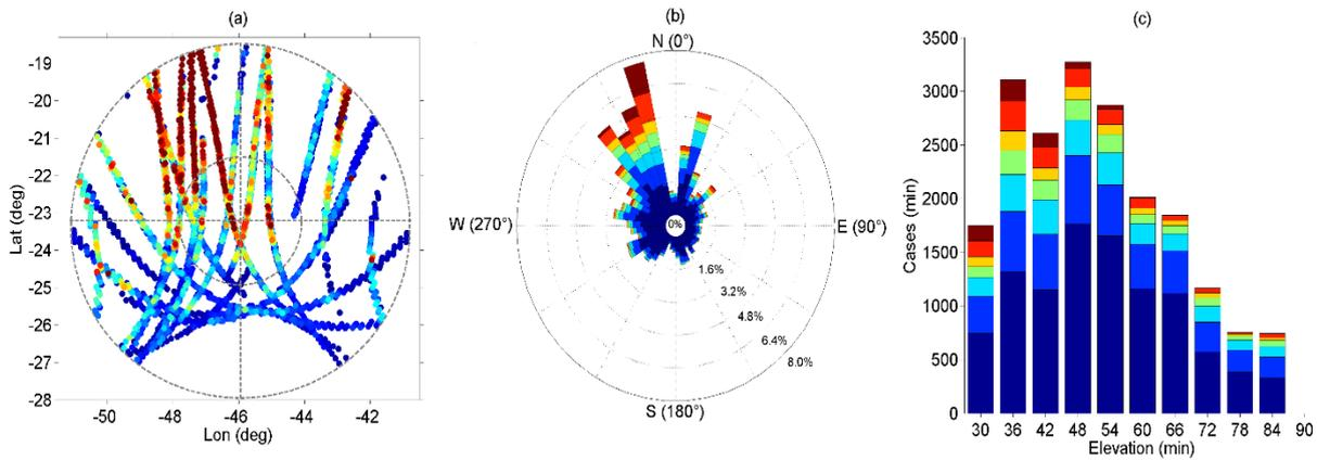
Figure 12: (a) The spatial distribution of amplitude scintillation events plotted at the respective IPP values for GPS-L1 signals. The outer and inner circles define elevations equal to 20° and 60°, respectively; (b) The statistical distribution of  $S_4$  as a function of azimuth. The  $S_4$  range groups for the azimuth and elevation plots share the same color code. (c) The statistical distribution of  $S_4$  as a function of elevation is shown as bar charts (source: the authors).
