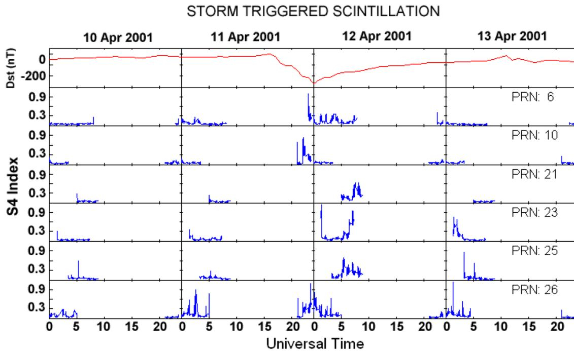
Figure 10: Example of storm scintillation triggering during the night of 11 to 12 of April 2001 under the effect of a strong magnetic storm. In the upper panel it is plotted the Dst index (source: the authors).
