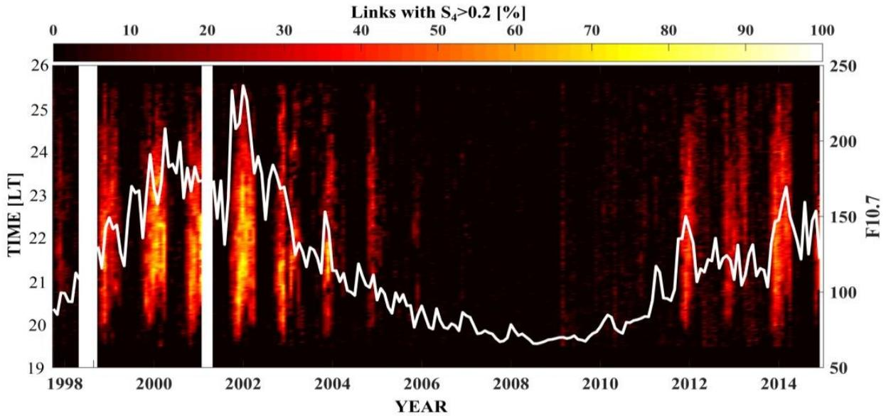
Figure 5:  $S_4$  data from the low-latitude GNSS receiver at Cachoeira Paulista and F10.7 cm solar flux (white continuous curve) from 1998 to 2014 (source: [de Paula et al., 2021a](#)).
