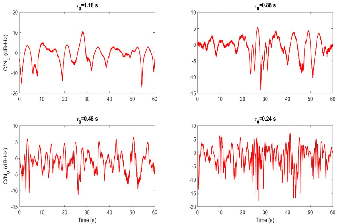
Figure 2: Amplitude scintillation patterns for almost the same  $S_4$  value ( $S_4 \sim 0.80$ ) but different decorrelation time  $\tau_0$  values (source: the authors).
