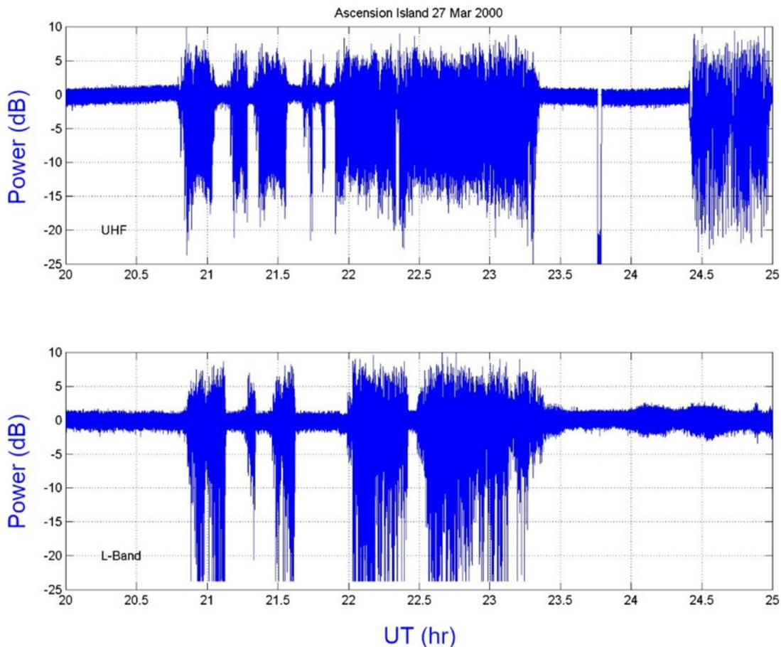
Figure 15: Simultaneous UHF (240 MHz) (upper panel) and L1 (1.575 GHz) (lower panel) from Ascension Island for March 27, 2000 (source: the authors).
