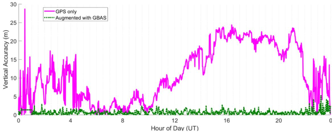
Figure 14: Vertical accuracy during field tests for GBAS Ground-Based Performance Monitor at Rio de Janeiro International Airport for November 13, 2011 (adapted from [Marini-Pereira et al., 2019](#))
