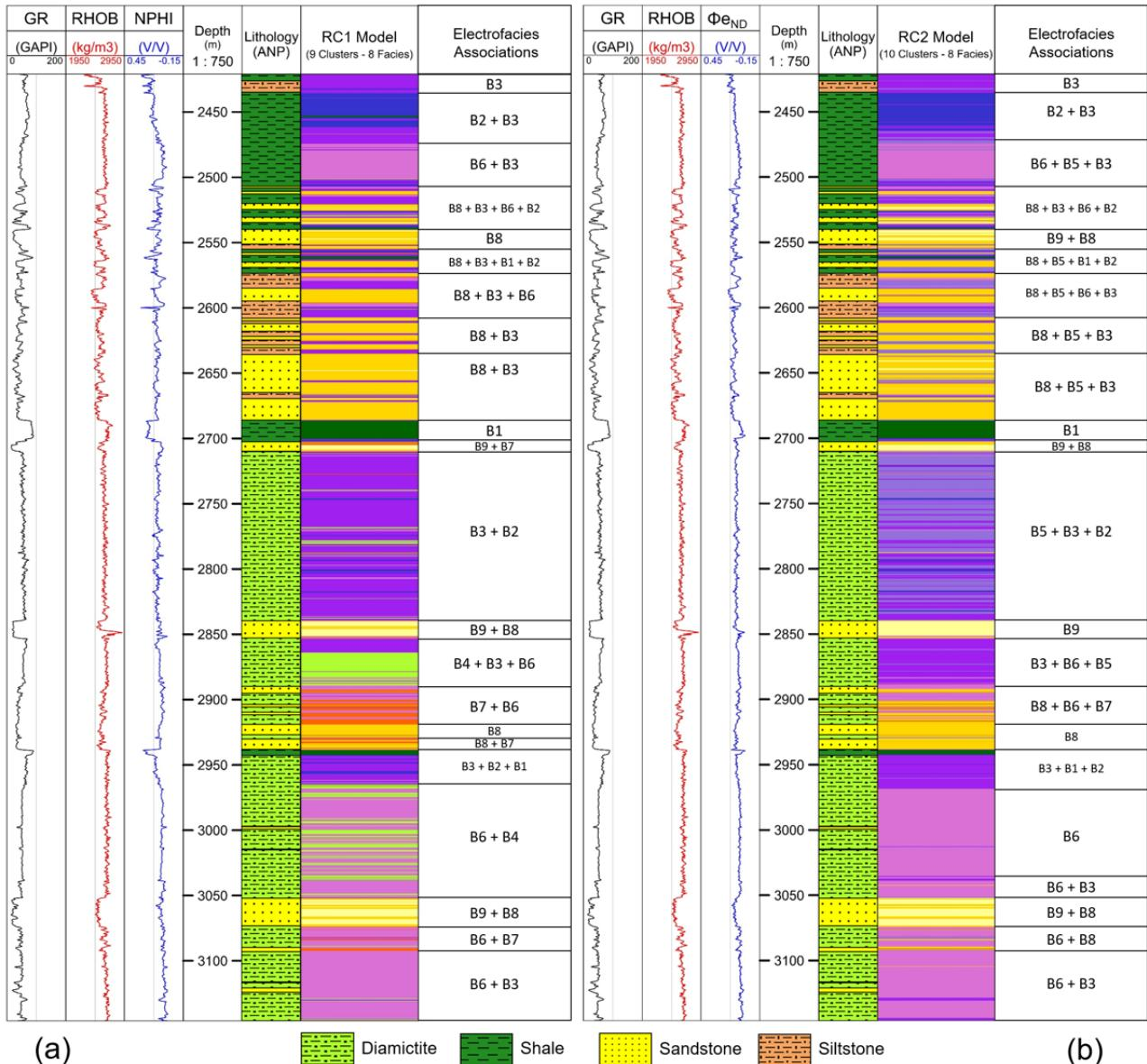
Figure 7: Models determined for well 1RCH-1-SC based on the neutron porosity log (a), and effective porosity determined by the neutron-density method (b).
