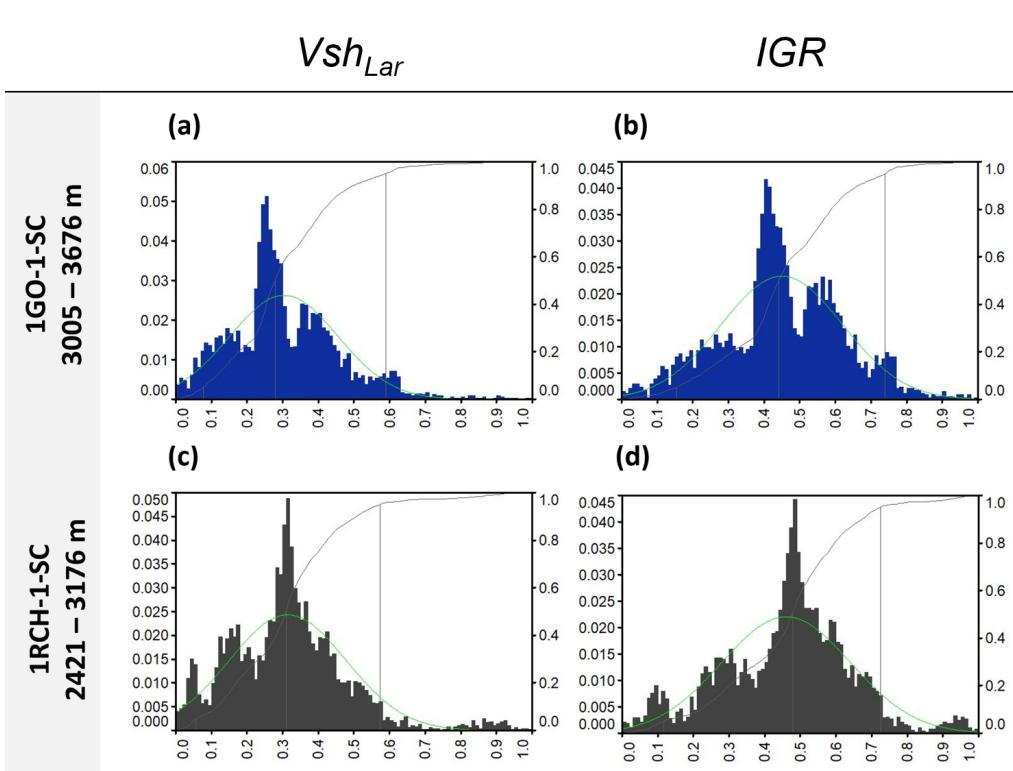
Figure 4: Comparative histograms of  $V_{sh}$  values determined by the Larionov method ( $V_{sh,Lar}$ ) and gamma ray index ( $IGR$ ) for wells 1GO-1-SC (a and b) and 1RCH-1-SC (c and d). Y axis (left side): frequency (fraction). Y axis (right side): accumulated fraction of data. X axis: volume shale (V/V). The depths are relative to the interval corresponding to the Itararé Group in the wells.
