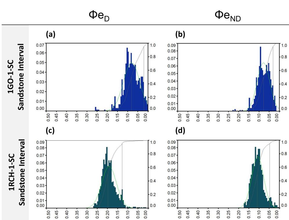
Figure 5: Comparative histograms of effective porosity values determined by the density method ( $\phi_{eD}$ ) and neutron-density method ( $\phi_{eND}$ ) for the sandstone interval of wells 1GO-1-SC (a and b) and 1RCH-1-SC (c and d). Y axis (left side): frequency (fraction). Y axis (right side): accumulated fraction of data. X axis: effective porosity (V/V).
