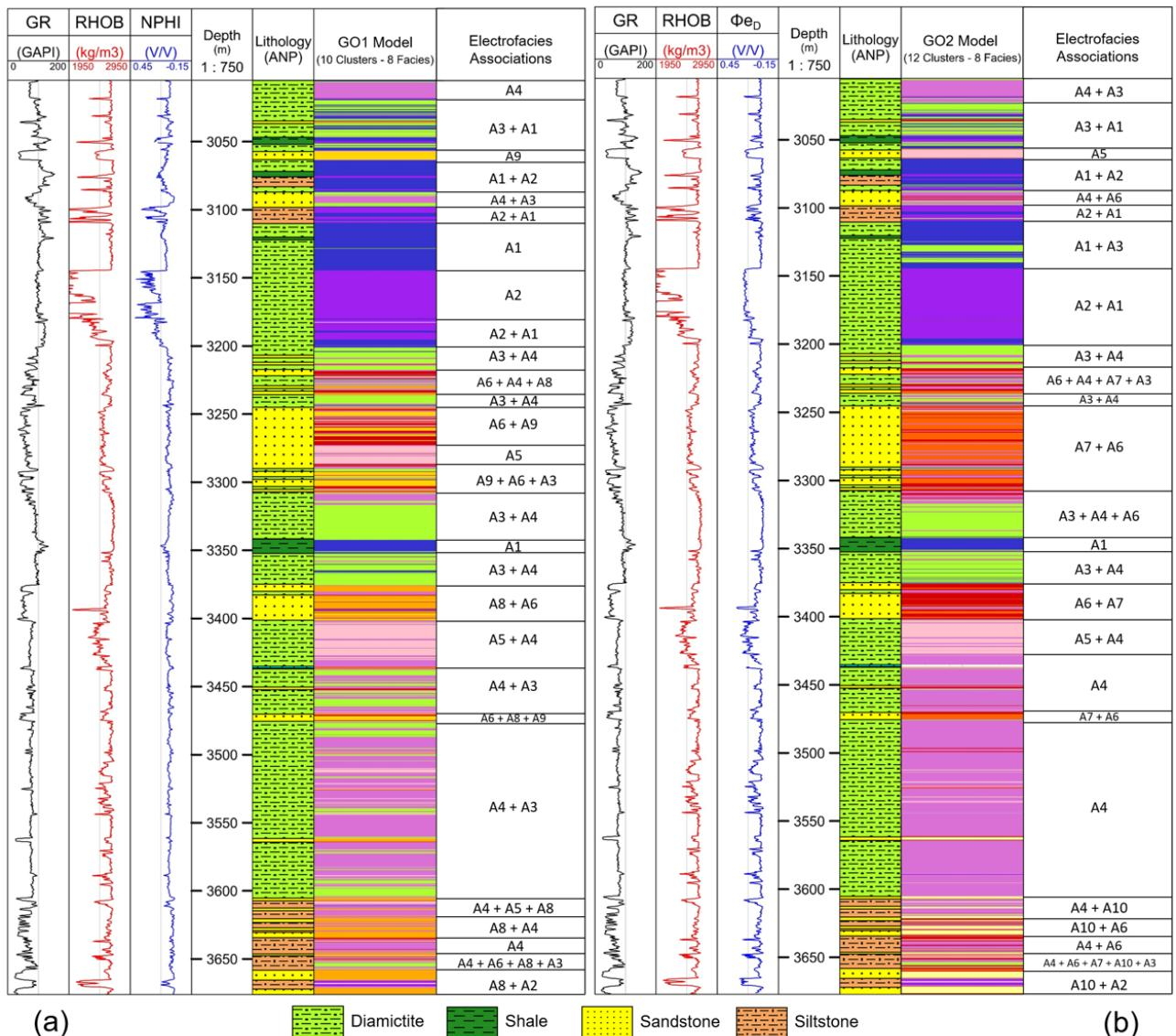
Figure 6: Models determined for the 1GO-1-SC well based on the neutron porosity log (a), and effective porosity determined by the density method (b).
