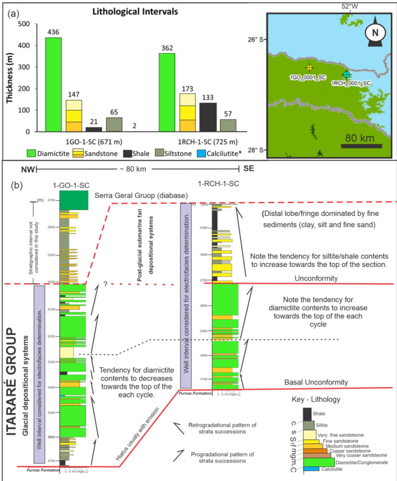
Figure 3: (a) Lithological intervals in wells 1GO-1-SC and 1RCH-1-SC: the lithological intervals represent the sum of all bed thicknesses of a given lithological unit. 671 m and 725 m are the sum of all interval thicknesses in each well. (b) Lithostratigraphic profiles from lithological data from each well.
