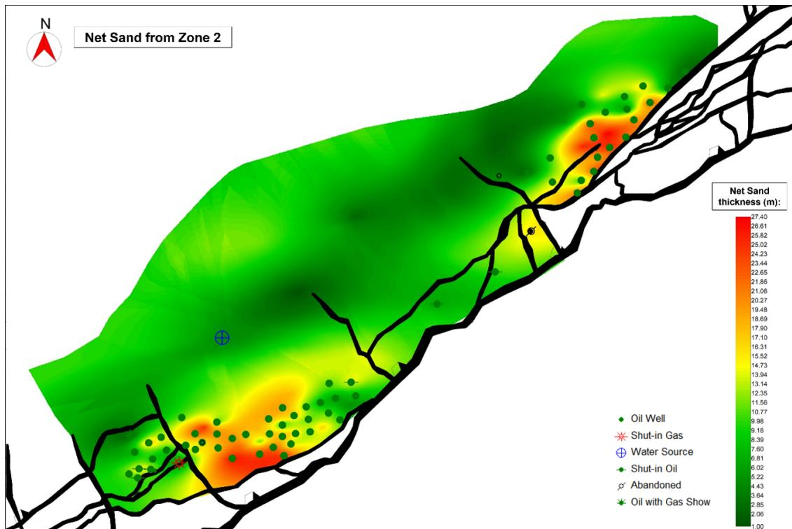
Figure 10: Isopach Net Sand Map coloured below the faults for the intermediary reservoir (Zone 2) generated using the cut-off of 10% for PHIE values and  $<50\%$  for Vsh. The well data were interpolated using the kriging geostatistical method. The portions with thicker net sand values are concentrated near the Carnaubais' Fault System showing a geometry very similar to alluvial fans. This figure was made using the S&P Kingdom software.
