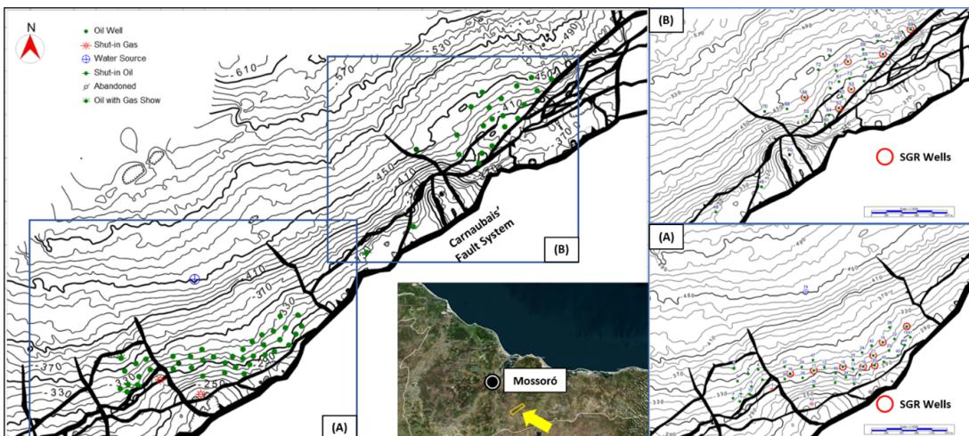
Figure 4: Location map of the study area in the southeastern portion of the Potiguar Basin. Wells with spectral gamma ray logs are highlighted in red. A) Group of wells in the southwestern area. B) Group of wells in the northeastern portion of the study area.
