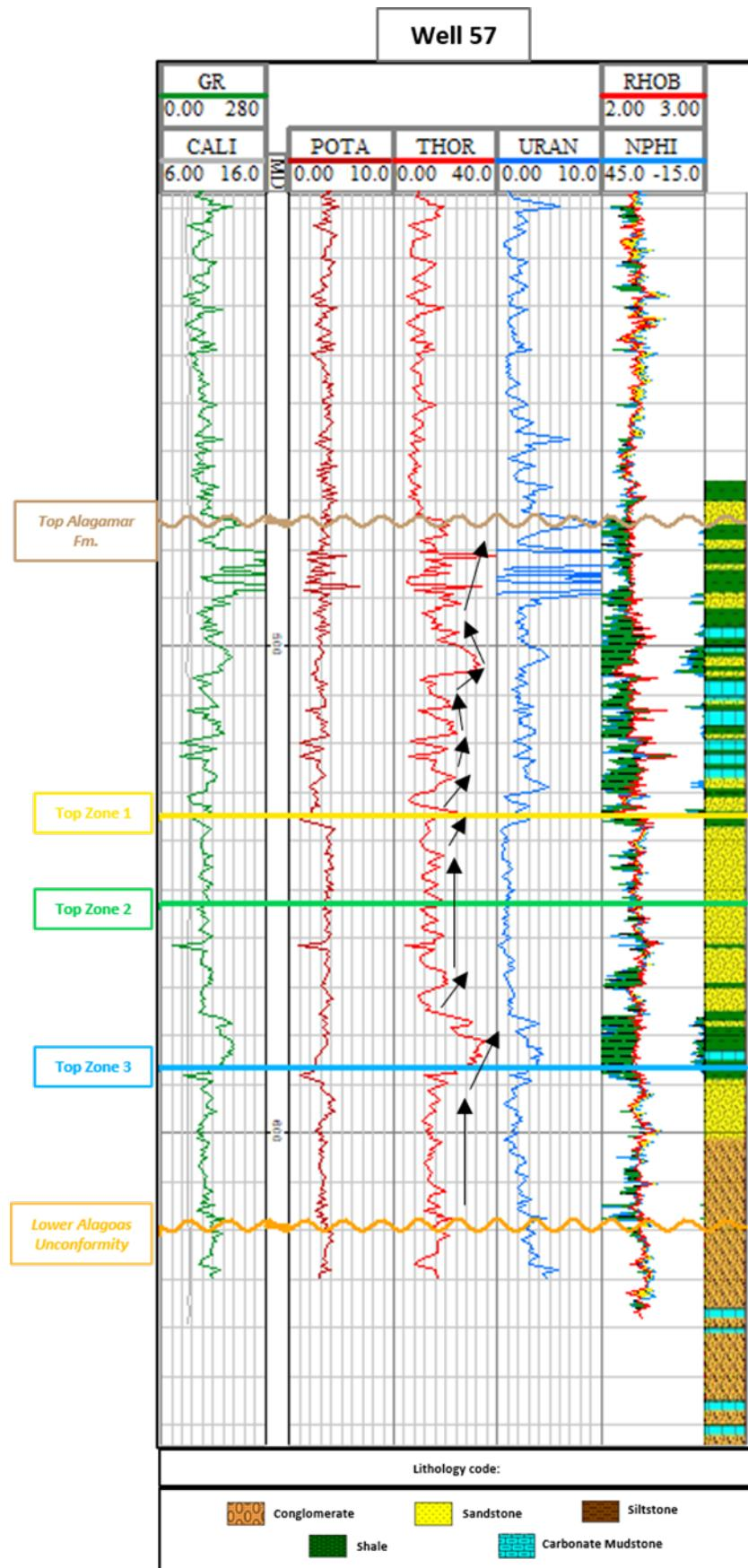
Figure 12: Composite log of the Well 57 showing the well tops interpreted. From track 1 to 7, the following logs are presented: CALI/GR, depth, Potassium (K - %), Thorium (Th - ppm), Uranium (U - ppm), NPHI/RHOB and mud logging description. The top and base of the Alagamar Fm. and the top of Zone 1 are well marked in the GR, NPHI and RHOB logs. However, the reservoir zone subdivision requires radioactive concentration logs together with the conventional ones.
