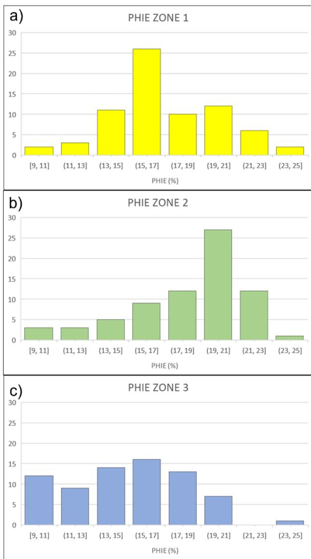
Figure 8: Histograms of effective porosity calculated for all the wells in the study area: (a) PHIE ZONE 1 - histogram for the top reservoir zone; (b) PHIE ZONE 2 - histogram for the intermediary zone; and (c) PHIE ZONE 3 - histogram for the basal zone.
