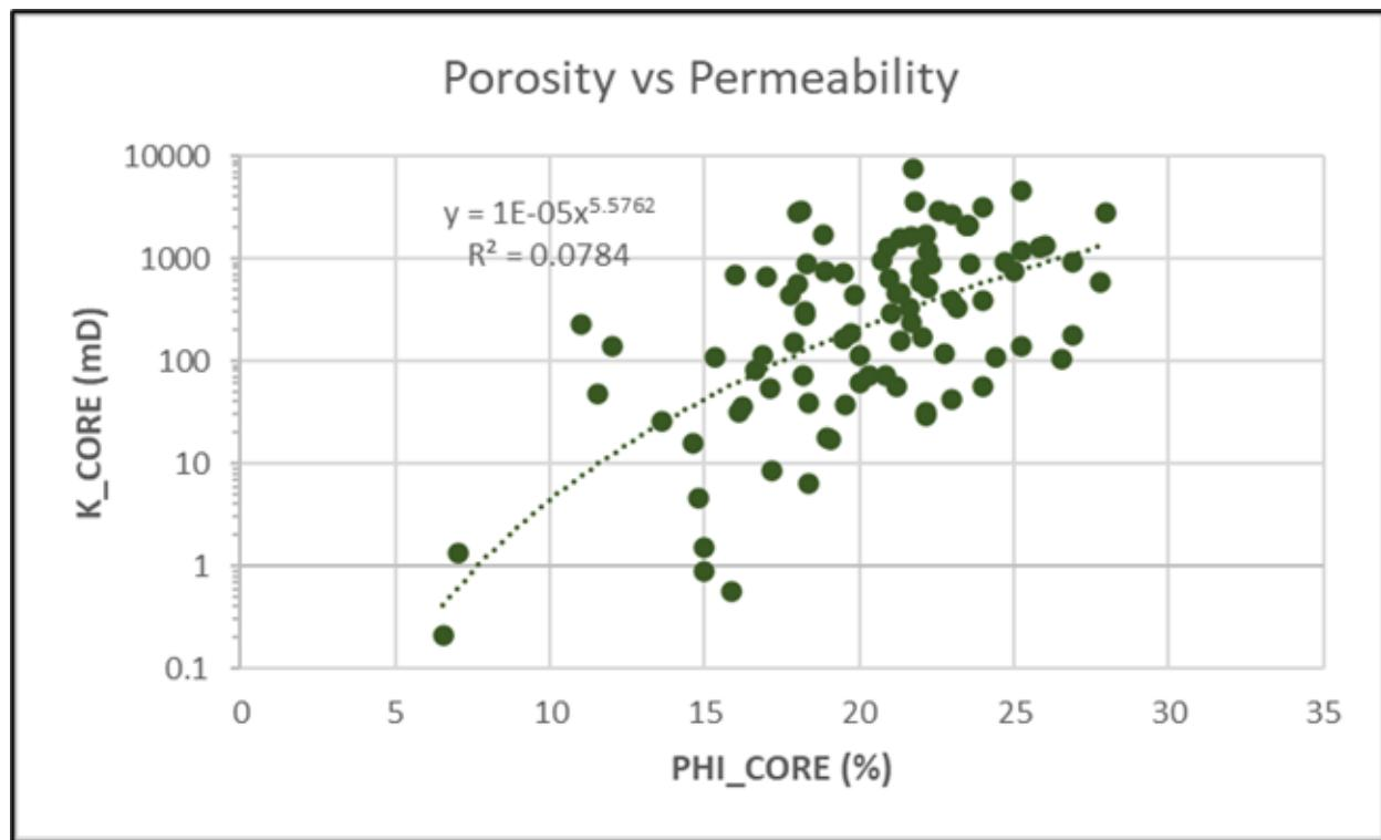
Figure 5: Correlation between the petrophysical laboratory measurement of effective porosity in 94 plug samples in four wells (PHI\_CORE) and the permeability (K\_CORE) also measured in these samples.
