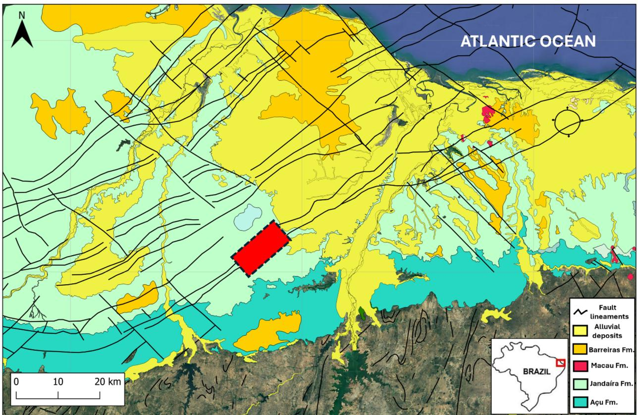
Figure 1: Regional Potiguar Basin showing the studied area (red rectangle) and the regional fault lineaments (in black). The Neogene rocks and deposits, the Açu and Jandaíra formations, crop out in the onshore section of the basin (modified from [Bertani et al., 1990](#); [Angelim, 2006](#); [De Castro and Bezerra, 2015](#)).
