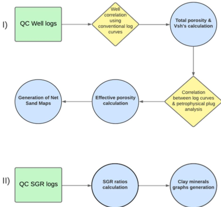
Figure 6: I) Workflow for the petrophysical evaluation and stratigraphic correlation between the reservoir zones; II) Workflow for the SGR log evaluation aiming a better clay mineral characterization.
