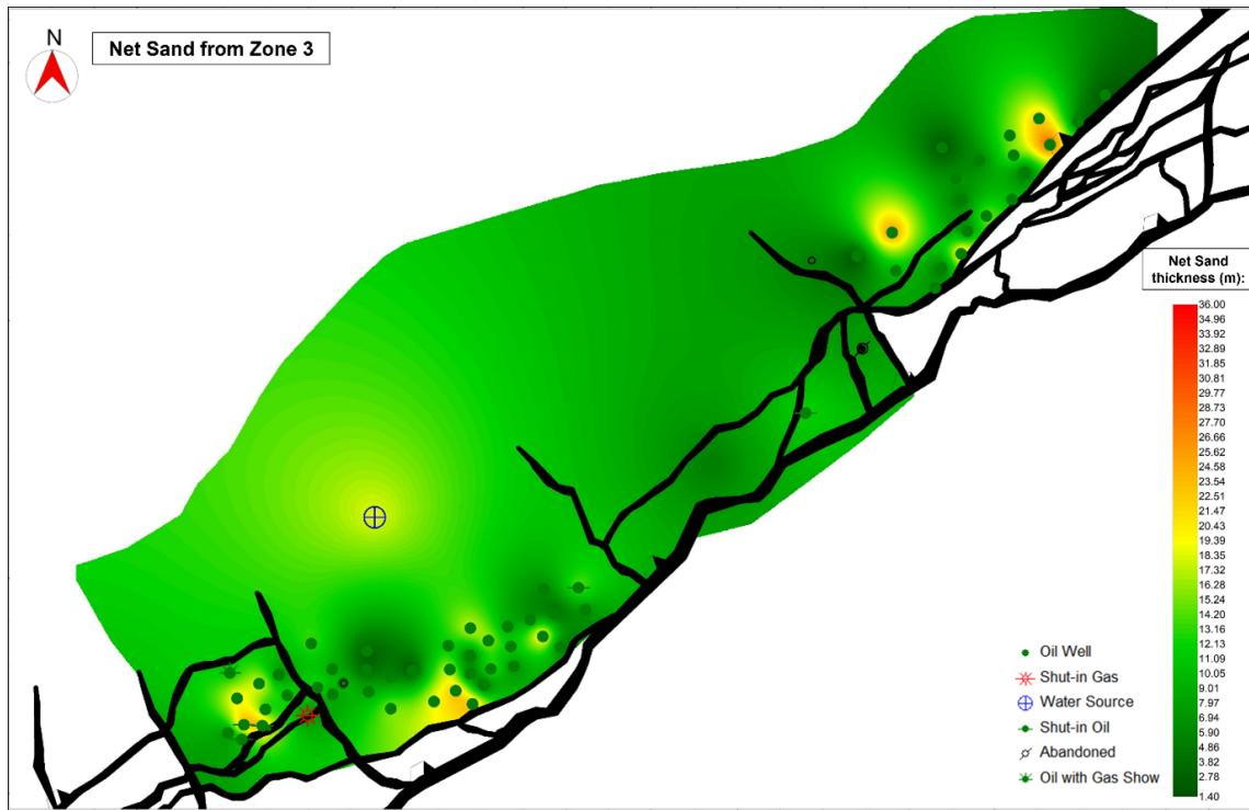
Figure 9: Isopach Net Sand Map colored below the faults for the basal reservoir (Zone 3) generated using the cut-off of 10% for PHIE values and  $<50\%$  for Vsh. The well data were interpolated using the kriging geostatistical method. The thicker net sand values seem to go basinward, in the northwestern direction. This figure was made using the S&P Kingdom software.
