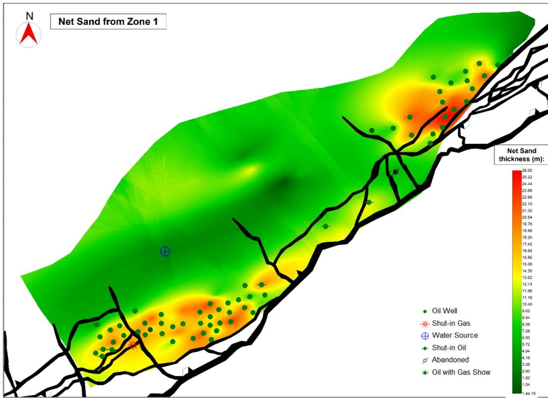
Figure 11: Isopach Net Sand Map coloured below the faults for the top reservoir (Zone 1) generated using the cut-off of 10% for PHIE values and  $<50\%$  for Vsh. The well data were interpolated using the kriging geostatistical method. The portions with thicker net sand values are concentrated near the Carnaubais' Fault System, like the intermediary zone map, but with a better lateral continuity parallel to this fault system. This figure was made using the S&P Kingdom software.
