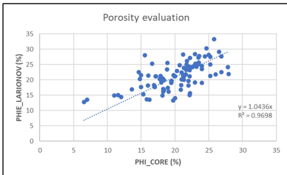
Figure 7: Correlation between the petrophysical laboratory measurement of the effective porosity in 94 plug samples in four wells (PHI\_CORE) and the effective porosity calculated using the Larionov Paleogene Rock method (PHIE\_LARIONOV).
