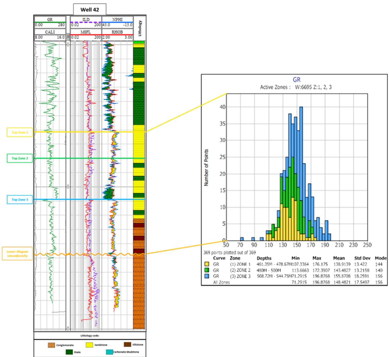
Figure 3: Well 42 with GR/CALI in track 1; ILD/MSFL in track 2; NPHI/RHOB in track 3; and mud logging in track 4. On the right, there is the histogram of GR values colored by the respective zone color (Zone 3 in blue; Zone 2 in green; and Zone 1 in yellow).
