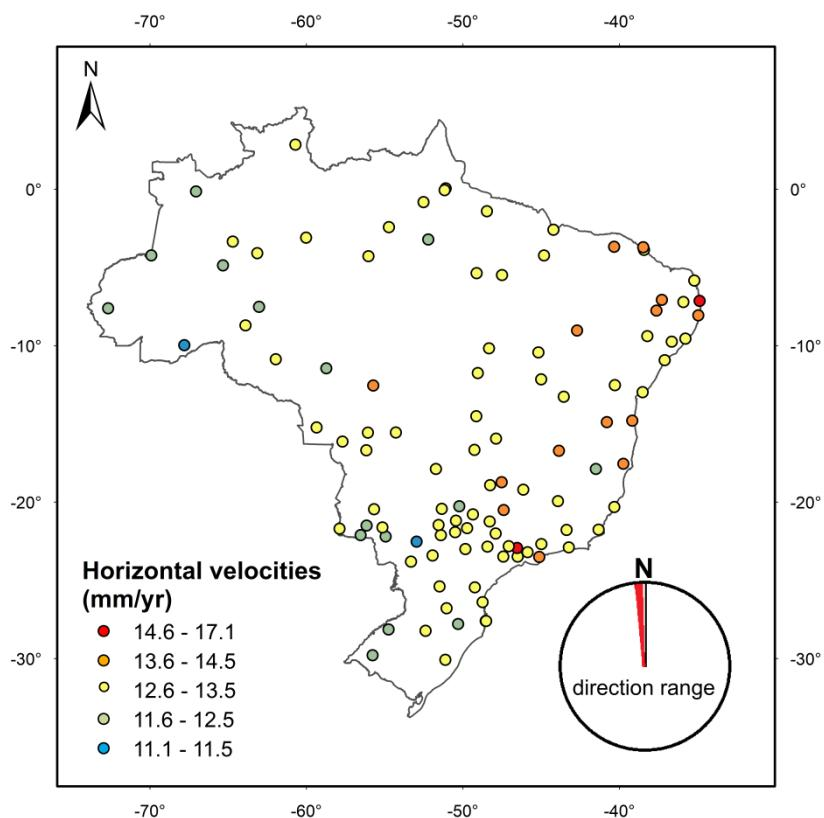
Figure 6: GNSS horizontal velocity model. The noise model used combines white noise and flicker noise.
