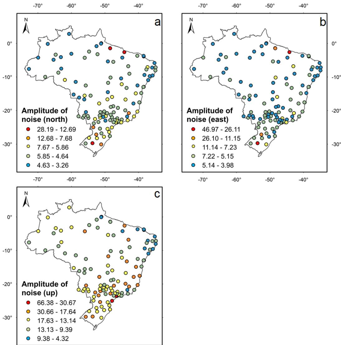
Figure 3: WN+RW noise amplitude, expressed as  $\text{mm} \times \text{year}^{-1/2}$ , in the north (a), east (b) and up (c) components.
