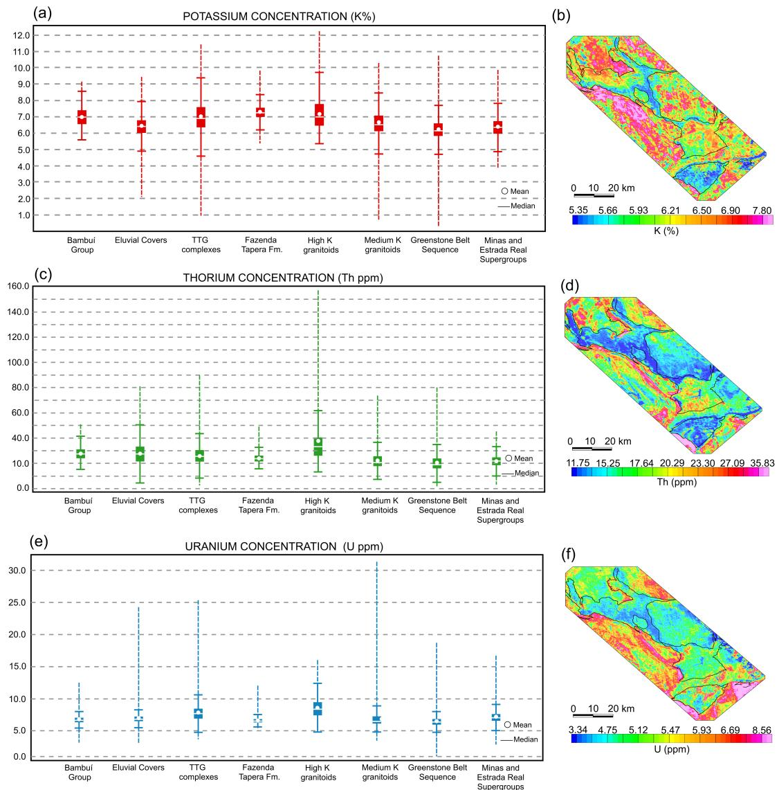
Figure 5: Boxplot graph of K, Th and U concentrations and their respective maps. (a) Boxplot of K (%) concentrations. (b) Radiometric map of the K (%) concentration. (c) Boxplot of Th (ppm) concentrations. (d) Radiometric map of the Th (ppm) concentration. (e) Boxplot of U (ppm) concentrations. (f) Radiometric map of the U (ppm) concentration.
