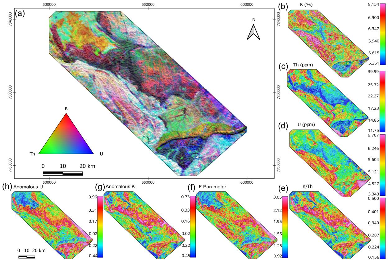
Figure 6: (a) RGB of K, Th and U ternary composition. (b) K concentration map (%). (c) Th concentration map (ppm). (d) U concentration map (ppm). (e) K/Th ratio map. (f) F Parameter map. (g) Anomalous K map ( $K_d$ ). (h) Anomalous U map ( $U_d$ ).
