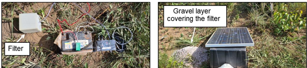
Figure 5: Typical installation of one of the temporary elements: Left – RS&Boom connected to the battery and filter; Right – Protective box for the equipment, a layer of gravel covering the filter and a solar panel.
