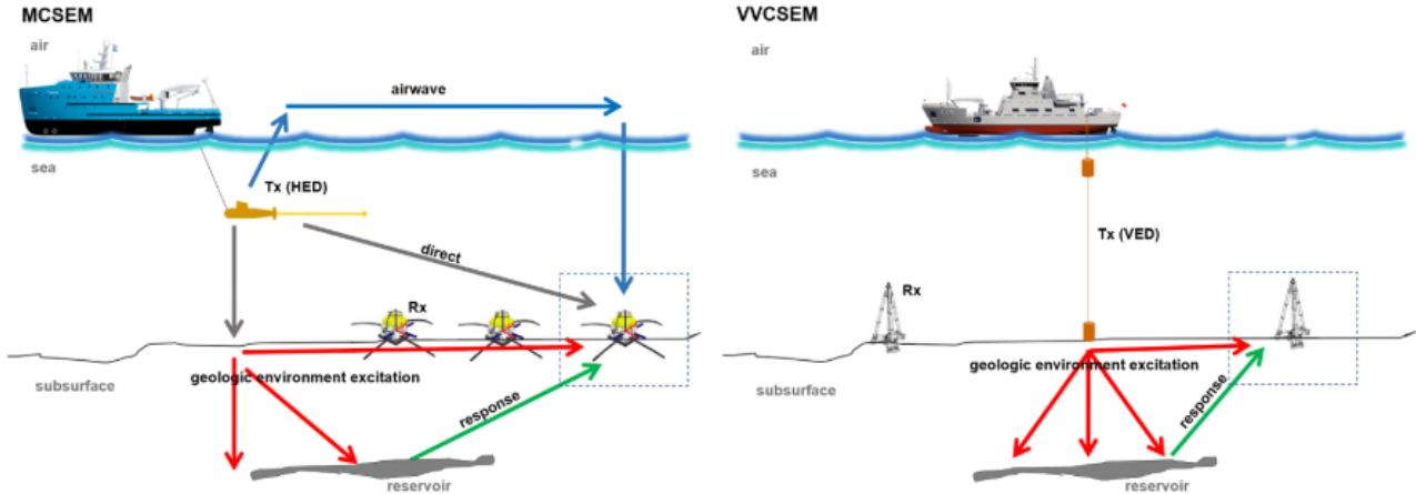
Figure 1: Comparative illustration of the MCSEM and VVCSEM methods. The blue line represents the airwave; the gray, the direct pulse of the  $Tx$ ; the red, the geologic environment excitation by the  $Tx$ ; and the green, the response of the interaction between the subsurface and the electric field produced by the source and the reservoir.
