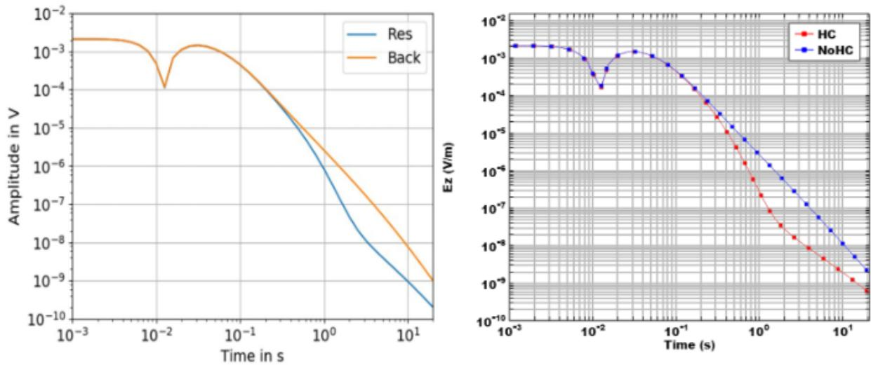
Figure 3: Comparison of the VVCSEM response (1D) from Holten et al. (2009) and Helwig et al. (2019) (left) with the response found with the 3D model in the multiphysics modeler (right), for the canonical model and 200 m offset.
