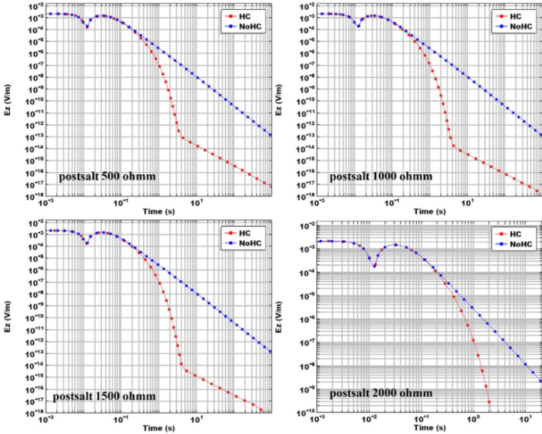
Figure 7: VVCSEM response for variation in the postsalt reservoir for electrical resistivity values of 500 Ohm.m, 1000 Ohm.m, 1500 Ohm.m and 2000 Ohm.m (seen from left to right and from top to bottom).
