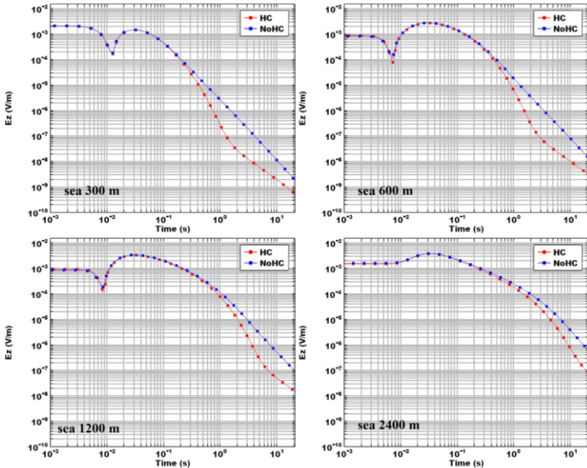
Figure 4: VVCSEM response for the 300 m, 600 m, 1200 m and 2400 m thick water slide (seen from left to right and from top to bottom).
