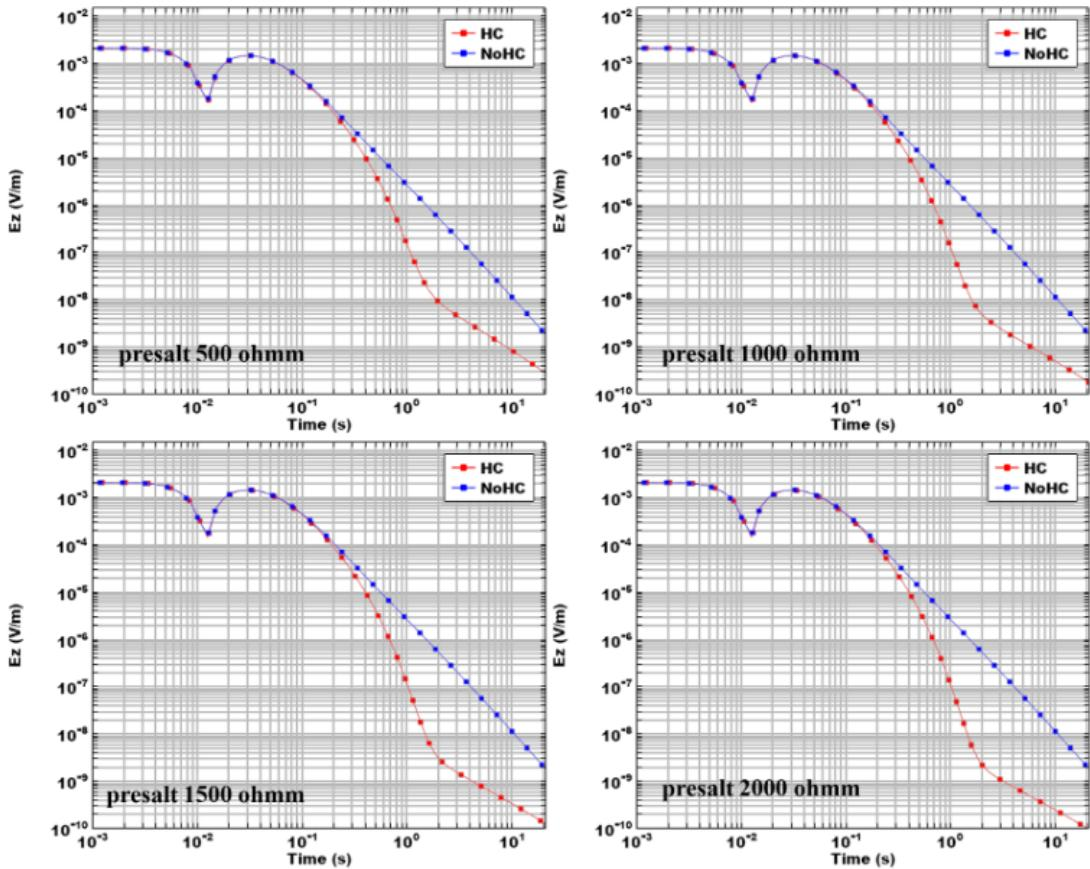
Figure 8: VVCSEM response for variation in the presalt reservoir for electrical resistivity values of 500 Ohm.m, 1000 Ohm.m, 1500 Ohm.m and 2000 Ohm.m (seen from left to right and from top to bottom).
