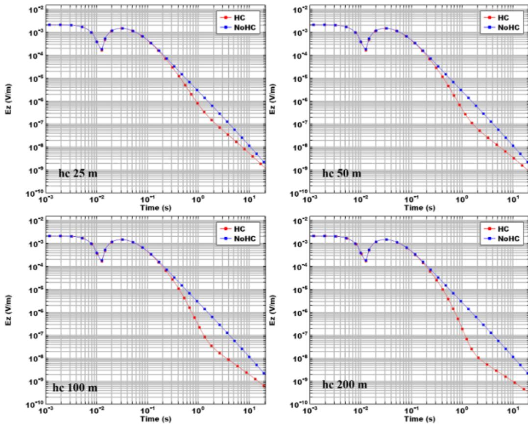
Figure 5: VVCSEM response for reservoir thickness values of 25 m, 50 m, 100 m and 200 m (seen from left to right and from top to bottom).
