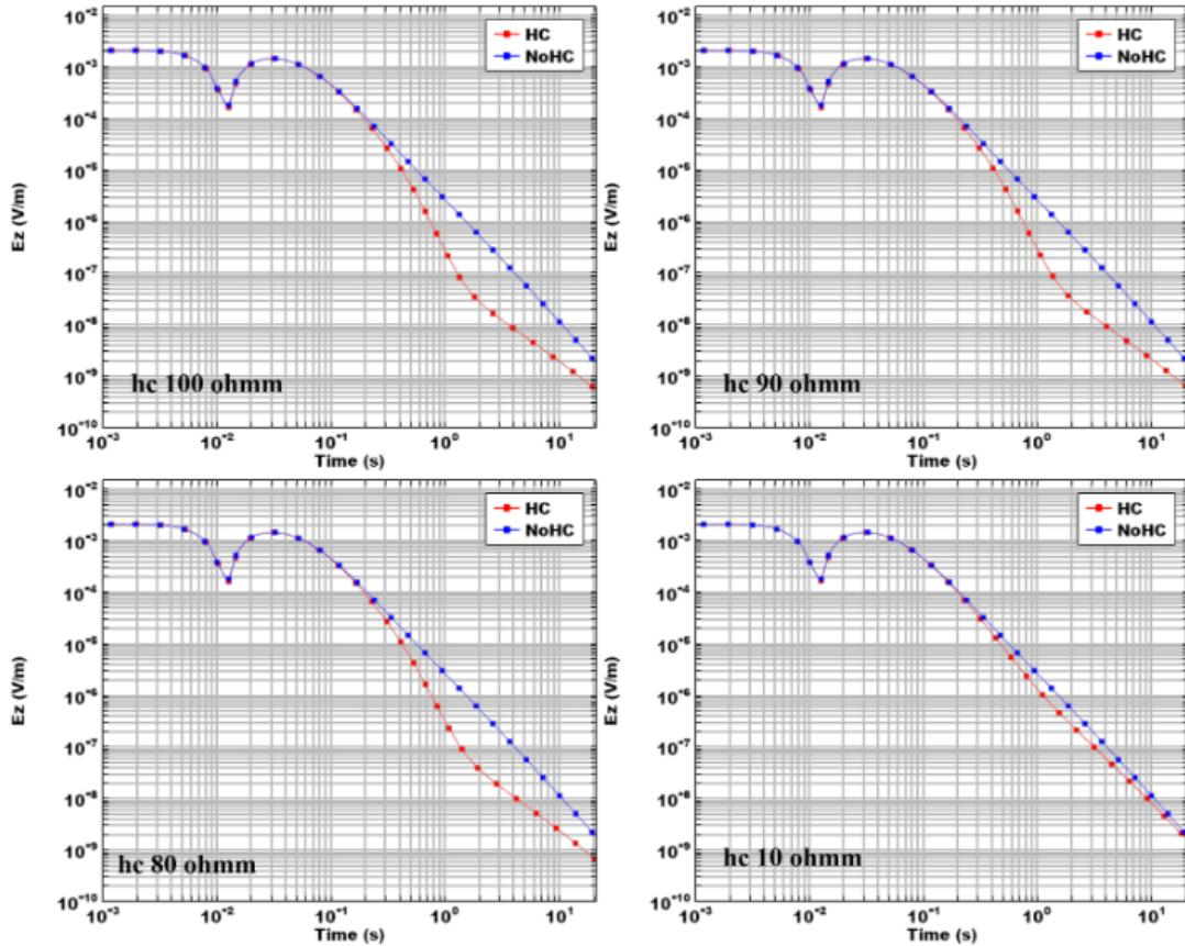
Figure 6: VVCSEM response for variation of electrical resistivity of the reservoir with values of 100 Ohm.m, 90 Ohm.m, 80 Ohm.m and 10 Ohm.m (seen from left to right and from top to bottom).
