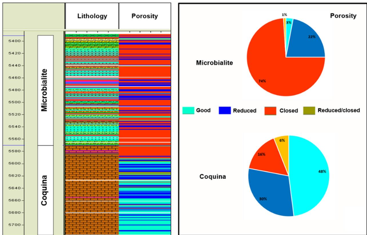
Figure 2: Porosity log next to the facies log. The porosity proportions can be compared between microbialite and coquina, where coquina is observed to be more porous. (Adapted from Silva et al., 2017.)
