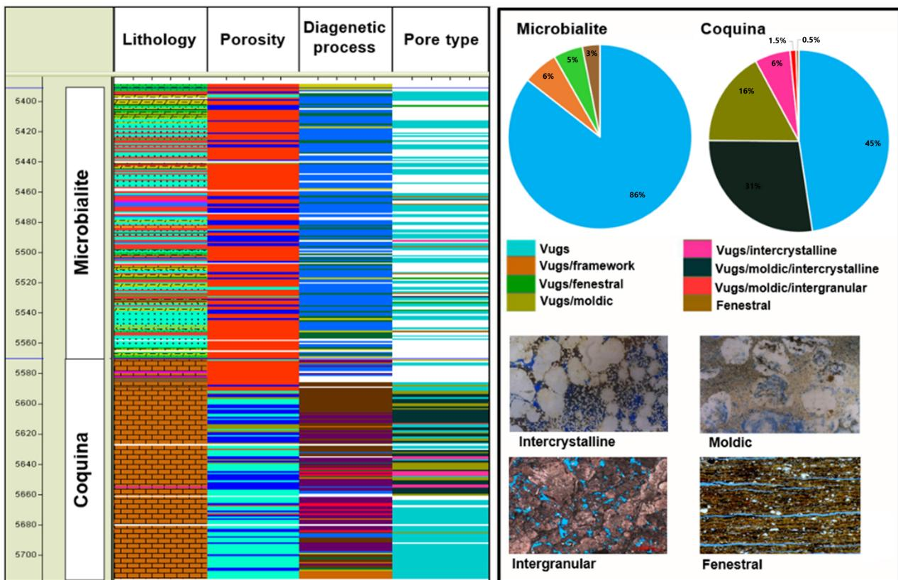
Figure 4: Pore type log next to the facies, porosity, and diagenetic process logs. Note in the pore type proportion graph and in its log that the vug type is predominant in microbialite and coquina. (Adapted from Silva et al., 2017.).
