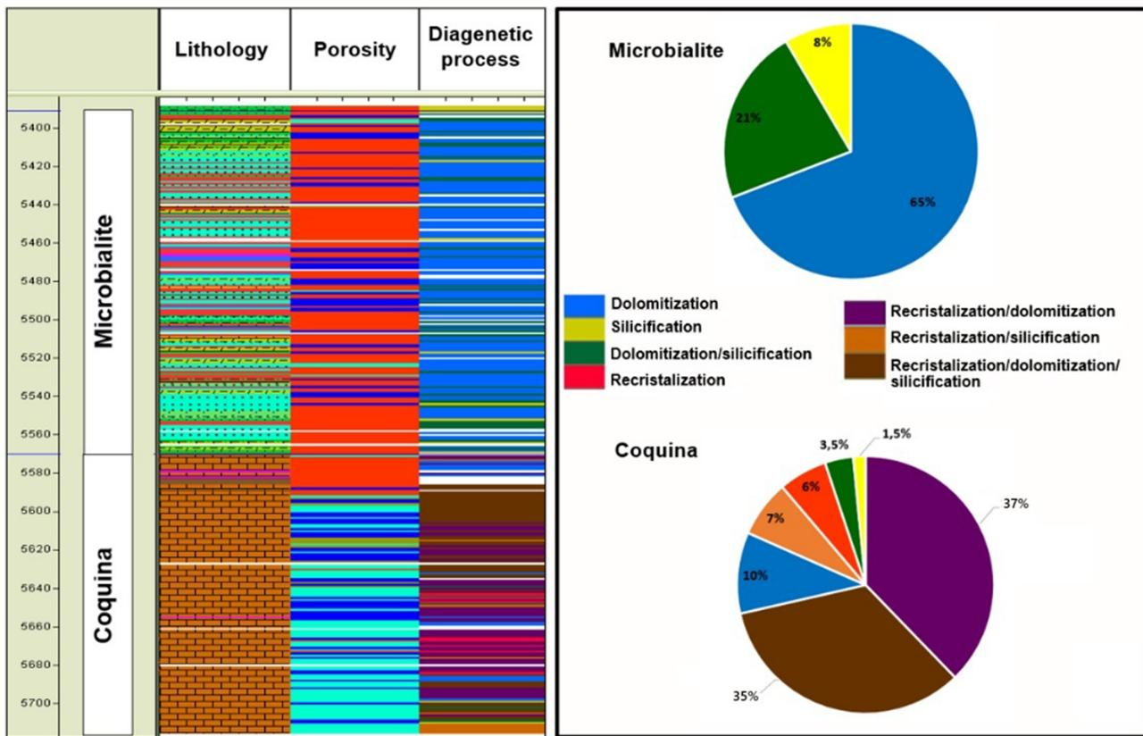
Figure 3: Diagenetic process log next to the facies and porosity logs. It is observed that dolomitization was the dominant process in microbialite, while in coquina it is combined with the recrystallization process. (Adapted from [Silva et al., 2017](#).)
