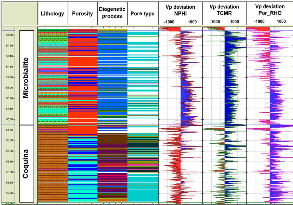
Figure 8: Facies logs - lithology, porosity, diagenetic process and pore type; and deviations of the P-wave velocity of the three porosities: NPHI, TCMR and Por\_RHO. The positive deviation is shown in blue hatching while the negative deviations are shown in red hatching.
