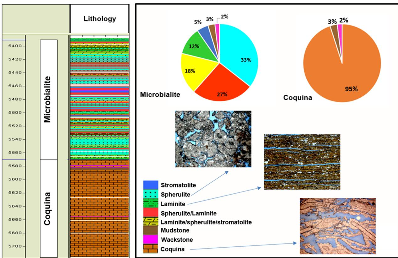
Figure 1: Facies log of lithology showing microbialite and coquina composition in the studied well. Note the predominance of laminite and spherulite in the microbialite. (Adapted from Silva et al., 2017).
