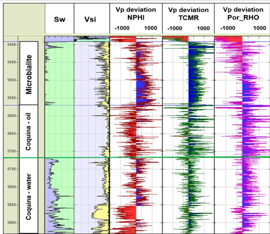
Figure 7: Logs of water saturation (Sw) (in faded blue), silica volume (Vsi) (in yellow) and velocity deviations of the P-wave of the three porosities: NPHI, TCMR and Por\_RHO in the microbialite and coquina zones. The positive deviation is shown in blue hatching while the negative deviations are shown in red hatching.
