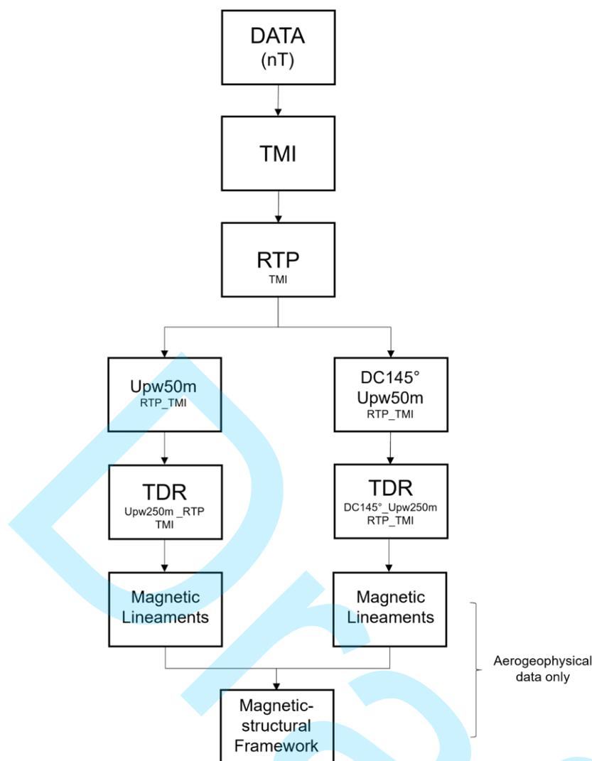
**Figure 3** – Aeromagnetic and magnetic data processing flowchart.
