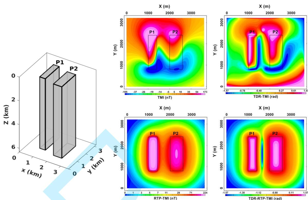
**Figure 2** – Synthetic model of prisms (P1 and P2) with dimensions of P1: 1 km (y) x 0.3 km (x) 6 km (z) starting at 100m of depth and P2: 1 km (y), 0.7 km (x) and 6 km (z) starting at 200m of depth and magnetic responses from synthetic data. Comparison between Total Magnetic Intensity (TMI), TDR\_TMI, RTP\_TMI and TDR\_RTP\_TMI anomalies.
