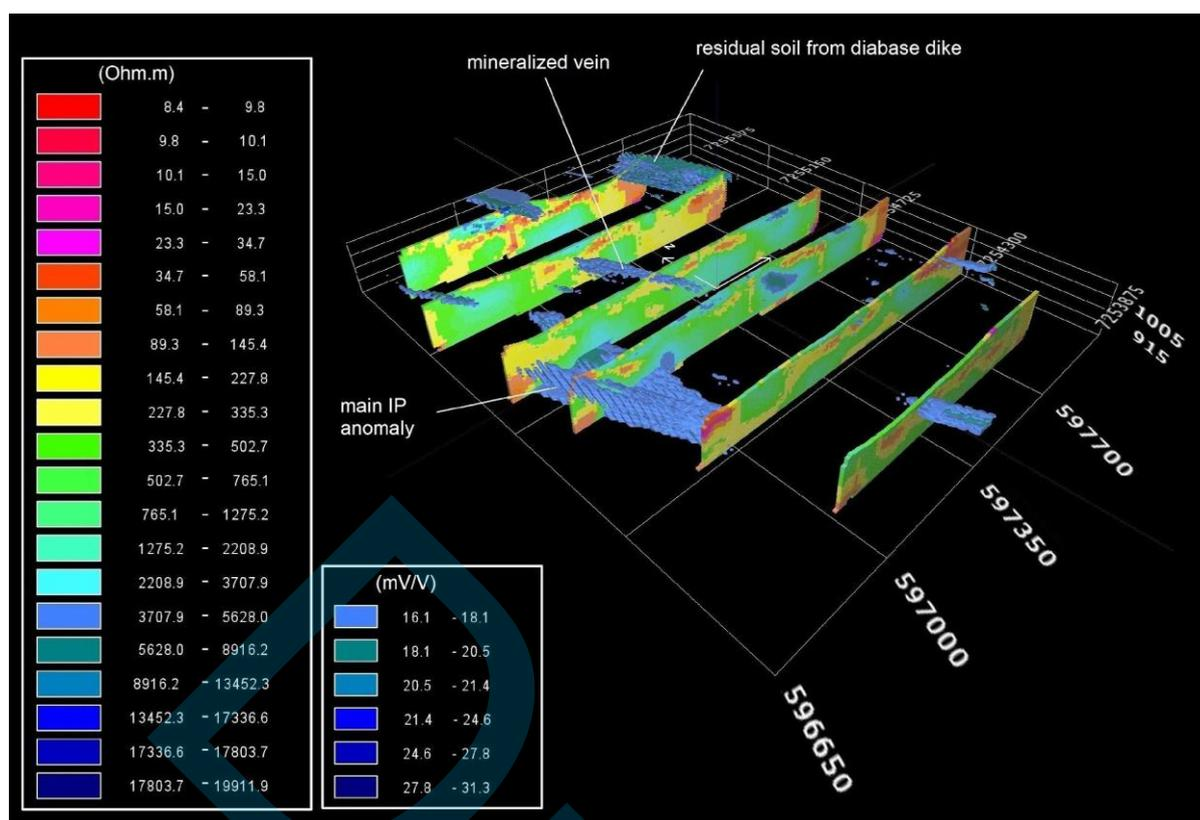
**Figure 9** – Voxel model with resistivity sections and chargeability volume. High values of IP are seen in conductive regions and an important anomaly is revealed in the center west.
