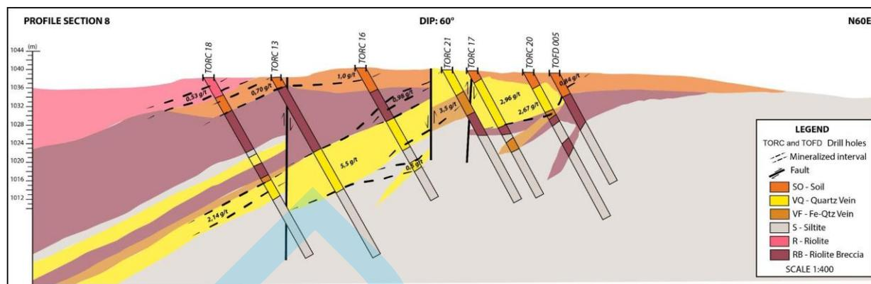
**Figure 11** – Geologic profile based on borehole data analysis. The drill core samples validates the geophysical models in the map section.
