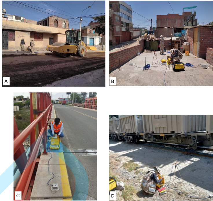
Figure 2: Photographs showing data acquisition along different sources: A) Compactor roller; B) Similar to scenario A, but with sensors installed on the roof of a two-story house in the district of Paucarpata; C) Vehicular traffic on bridges in the district of Socabaya; D) Railway transport near residential areas.
