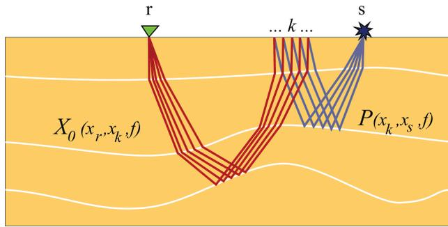
**Figure 7** – Diagram of how a first-order multiple for the 2D data are constructed. The multiple is a combination of a shot gather of the P data and a receiver gather of the primary impulse response  $X_0$ . These gathers are convolved and summed, generating the modeled multiple. Only one reflection from each wave field is shown (Verschuur, 2006).
