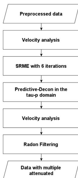
**Figure 13** – The combinations of methods that provide the best results: SRME and predictive deconvolution in the  $\tau - p$  domain followed by parabolic Radon filtering.
