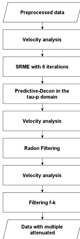
**Figure 14** – The combinations of methods that provide the best results: SRME and predictive deconvolution in the  $\tau - p$  domain followed by parabolic Radon filtering and  $f - k$  filtering.
