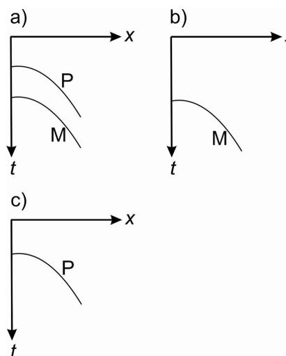
Figure 11 – Scheme of application SRME. a) Initially, the data are organized in families CMP in the field of acquisition. b) By the convolution original data with itself the multiple are modeled. c) The multiple modeled are subtracted from the original data and the residual data consist of primary reflections.
