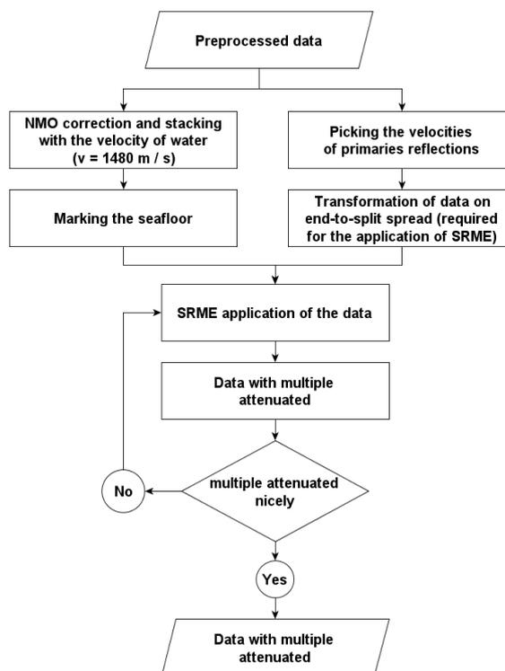
Figure 10 – Flow charts for the attenuation of surface multiples: SRME.
