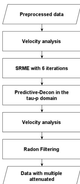
**Figure 13** – The combinations of methods that provide the best results: SRME and predictive deconvolution in the  $\tau - p$  domain followed by parabolic Radon filtering.
