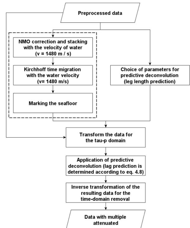
**Figure 6** – Flow charts for the attenuation of surface multiples: predictive deconvolution in the  $\tau - p$  domain.
