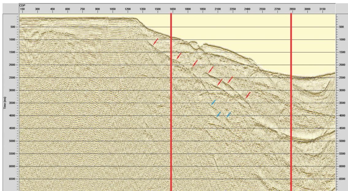
**Figure 12** – Raw seismic section organized by minimum offset (150 m) with gain (automatic gain control, AGC). The red and blue arrows indicate first- and second-order surface multiples, respectively. The solid orange lines represent the CMP gathers chosen for the analysis.
