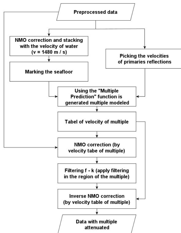
**Figure 2** – Flow charts for the attenuation of surface multiples:  $f - k$  filtering.
