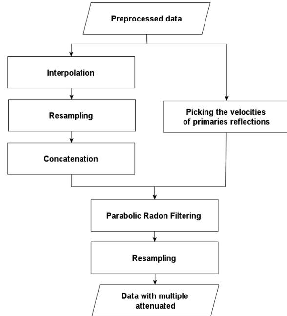
**Figure 4** – Flow charts for the attenuation of surface multiples: parabolic Radon filtering.
