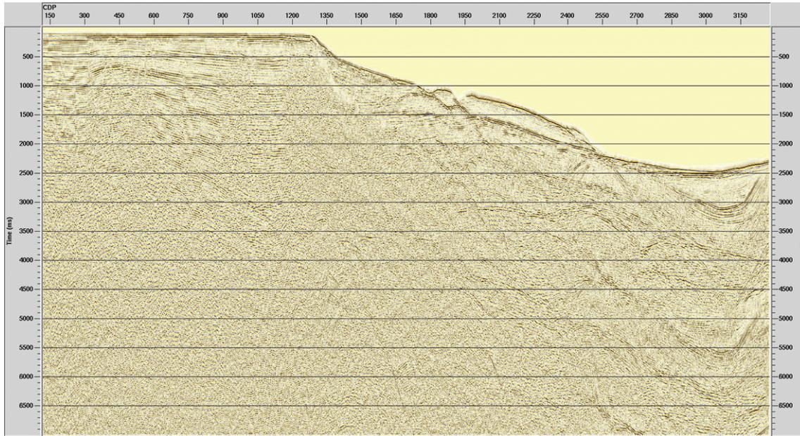
**Figure 17** – Data organized by minimum offset (150 m) with gain (AGC), after the application of SRME and predictive deconvolution in the  $\tau - p$  domain followed by parabolic Radon filtering.
