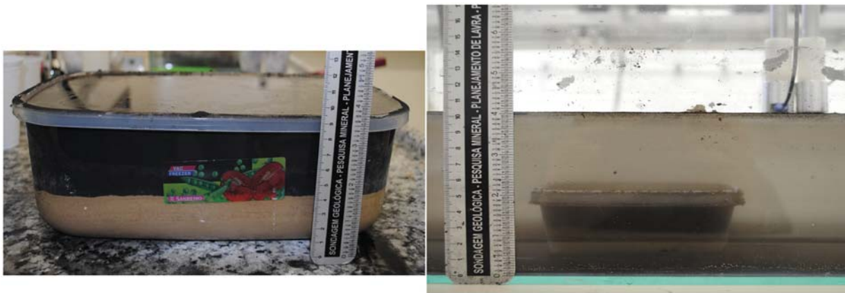
Figure 1 – Final aspect of the models. Model 1 (left) and model 2 (right). Model 2 is shown immersed in the water filled tank. In the upper right corner one can see the ultrasonic transducers. Note the zero offset of the transducers.
