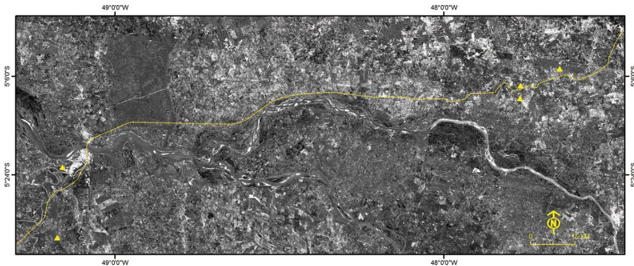
**Figure 7** – Mosaic of images from PC4 from the scenes/point orbit 222/63, 222/64, 223/63 and 223/64, generated from the principal components transform of the original TM 1–3–4–5 channels. The iron oxide minerals are enhanced as light regions. The continuous yellow line represents to the approximate position of the Carajás railroad. The yellow triangles correspond to known occurrences.
