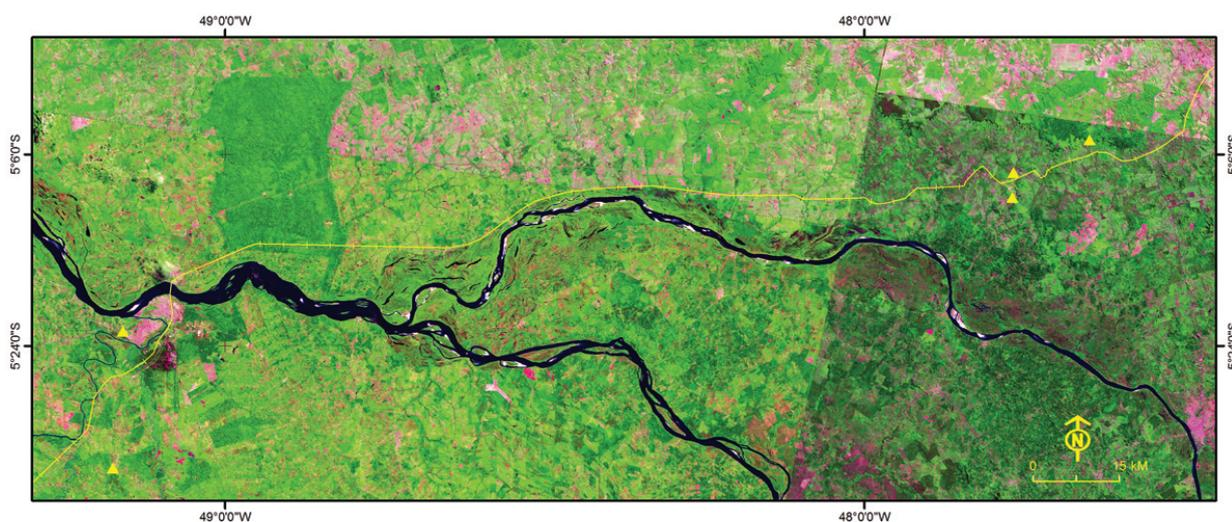
**Figure 6** – Color composition R5G4B3. The green color indicates vegetation (undifferentiated), the pink, is exposed soil and the magenta indicates urban areas. The continuous yellow line represents the approximate position of the Carajás Railroad. The yellow triangles correspond to the occurrence of catalogued lateritic crusts.
