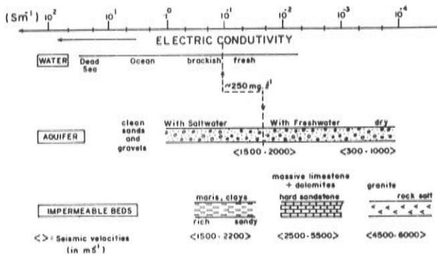
Figure 2 — Electrical conductivities of water, aquifer and impermeable beds (after Flathe, 1967).
