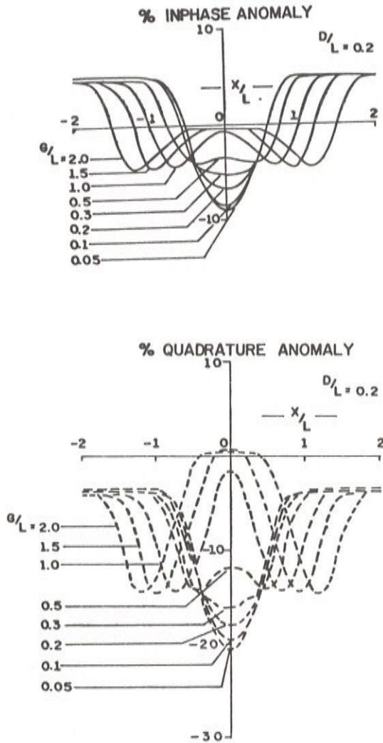
Figure 5 — Anomaly profiles over a resistive gap between graphite slabs for  $D/L = 0.2$ .
