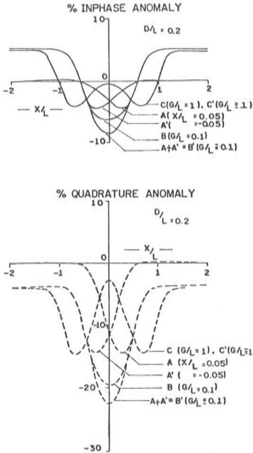
Figure 7 - Anomaly profiles for  $D/L = 0.2$ : A and A' due to the edges of a graphite slab positioned separately at  $X/L = 0.05$  and  $-0.05$ ; B and B' over the air-gap  $G/L = 0.1$ , B' being the combination of A and A'; and C and C' over the air-gap  $G/L = 1.0$ ; C' being the combined curve due to the edges positioned at  $X/L = 0.5$  and  $-0.5$ .
