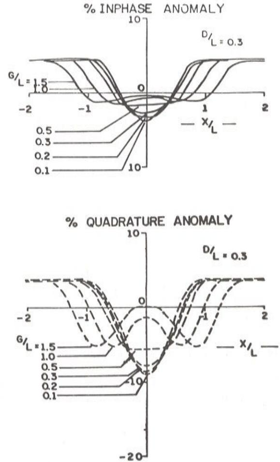
Figure 6 — Anomaly profiles over a resistive gap between graphite slabs for  $D/L = 0.3$ .
