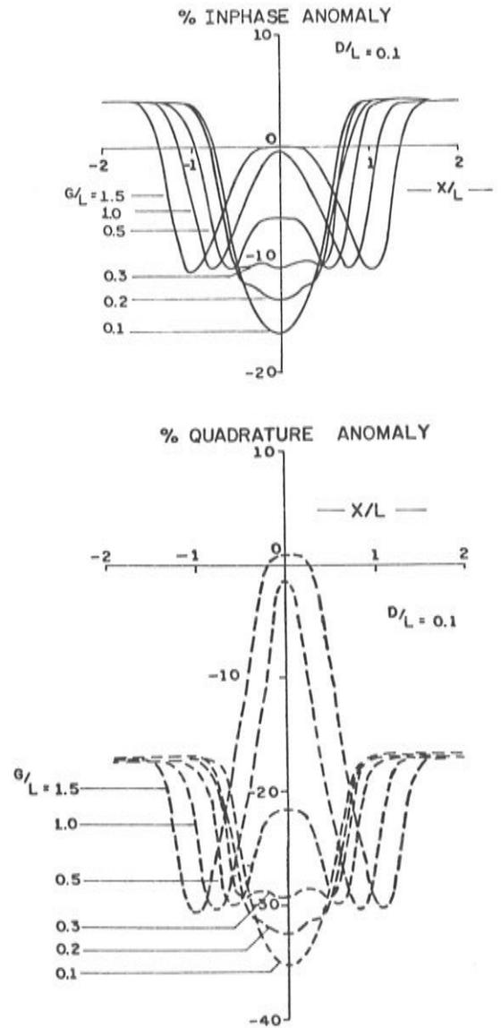
Figure 4 — Anomaly profiles over a resistive gap between graphite slabs for  $D/L = 0.1$ .
