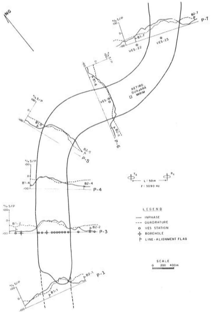
Figure 8 - Electromagnetic profiles across a buried stream channel "Guajará Mirim", Marajó Island, Brazil (After Porsani et al, 1980).
