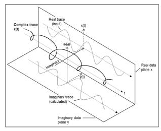
Figure 2: Representation of a complex seismic trace: real part x(t) and imaginary part y(t) that are added in a vector sense, resulting in the helical spiral z(t). After Hardage (2010).
