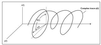
Figure 3: Instantaneous seismic attributes: the instantaneous amplitude a(t) is the magnitude of the vector perpendicular to the time axis that intersects the complex trace z(t); the instantaneous phase  $\Phi(t)$  is the angle that this vector makes with the real plane. The instantaneous frequency  $\omega(t)$  is determined by the rate of change of the instantaneous phase. After Hardage (2010).
