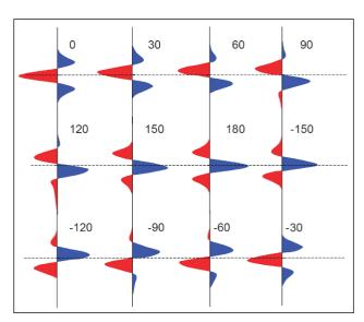
Figure 4: Phase change of a zero-phase wavelet. <u>Simm and White (2002)</u>.
