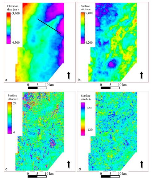
Figure 15: a) Reference surface in two-way time; b) compressional velocity; c) instantaneous phase; d) instantaneous frequency.
