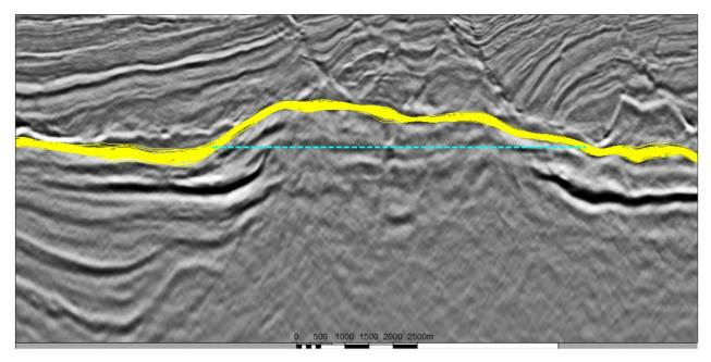
Figure 18: Seismic section with 100 surface realizations (yellow). The dashed blue line represents the considered oil-water contact.
