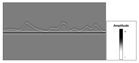
Figure 9: Synthetic seismic section, using zero-phase Ricker wavelet.
