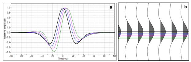
Figure 11: a) Wavelets used to generate synthetic seismic sections; b) Zero-phase seismic section in wiggle format and horizons picked in different phase rotation scenarios.
