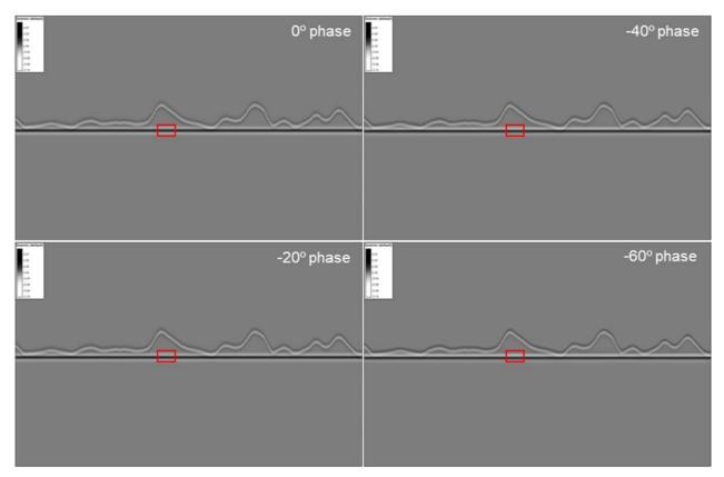
Figure 10: Synthetic seismic sections generated using wavelets with different phases. The red square represents the detailed area shown in <u>Figure 11b</u>.
